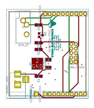
Spacing for the headers is board perfect, by aligning my grid, with the MSP430's design files grid (eagle), and making them align. FOSS+OSH win.
