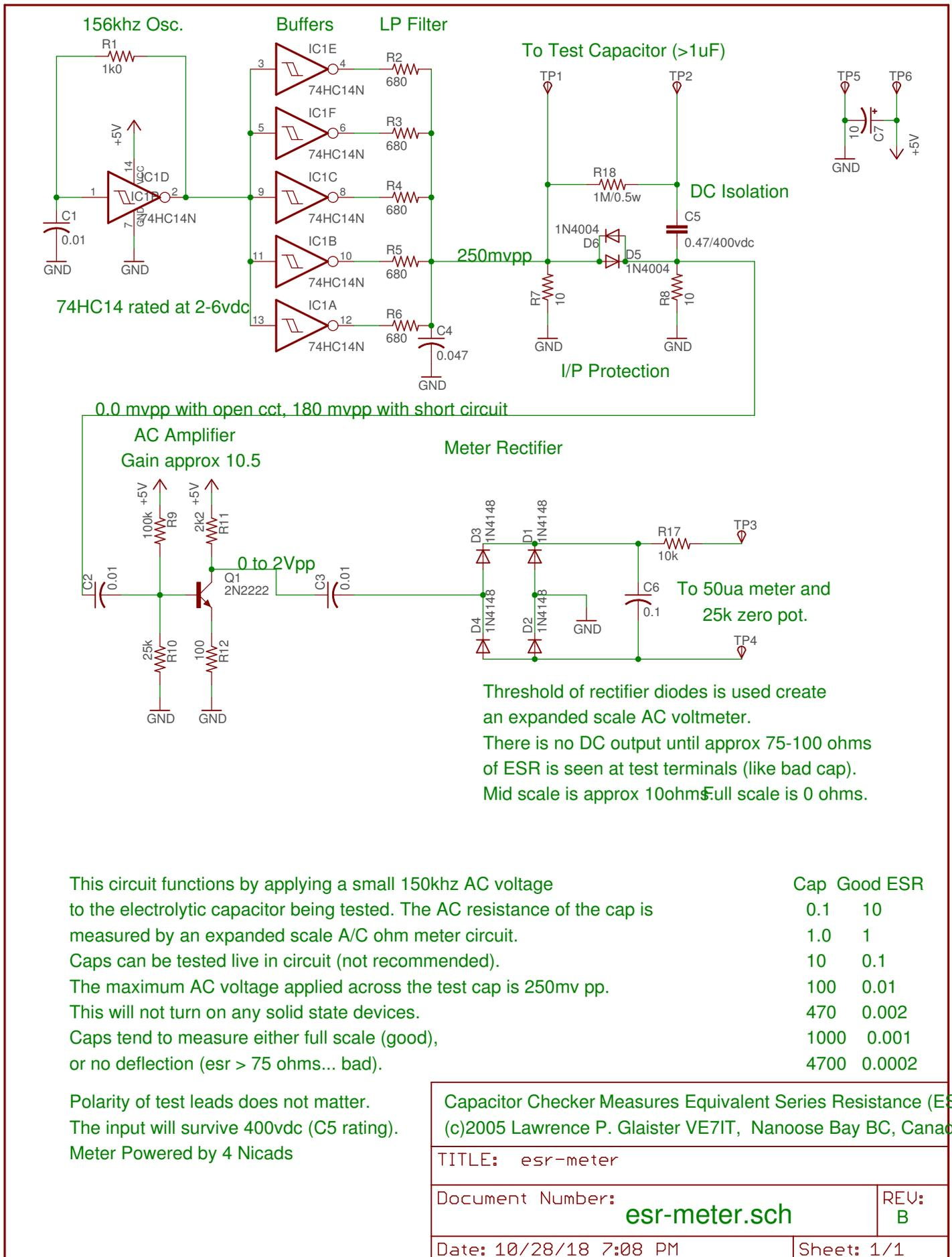
This circuit functions by applying a small 150kHz AC voltage to the electrolytic capacitor being tested. The AC resistance of the cap is measured by an expanded scale A/C ohm meter circuit. Caps can be tested live in circuit (not recommended). The maximum AC voltage applied across the test cap is 250mv pp. This will not turn on any solid state devices. Caps tend to measure either full scale (good), or no deflection (esr > 75 ohms... bad).
