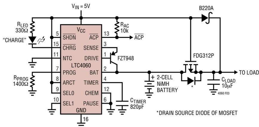
Figure 3. 1A Charger Application with Power Path Control
