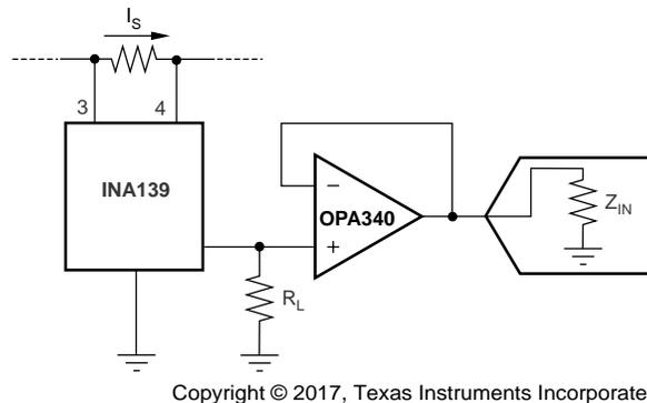
(1) Buffer of amp drives the A/D converter without effecting gain
