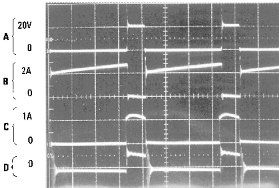
A: Switch pin voltage, 20 V/div
