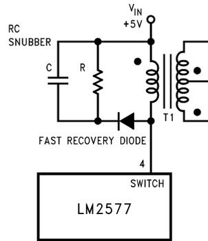
Figure 43. Snubber Circuit
