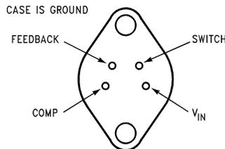
Figure 7. 4-Lead TO-220 (K) – Bottom View
