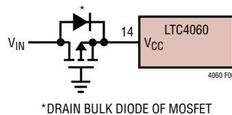
Figure 6. Low Loss Reverse Input Voltage Protection
