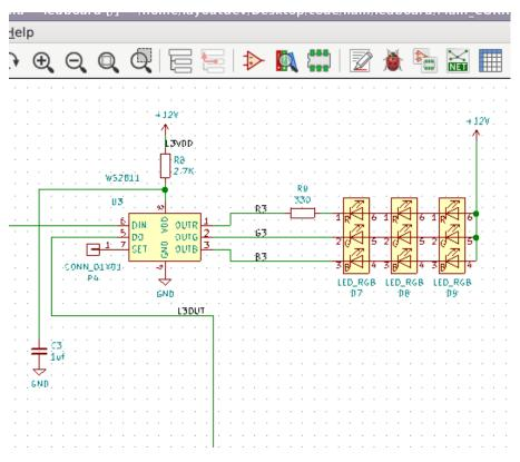
Adding net labels, makes line identification on layout easier. Here we have R3, B3, and G3, telling us that these leds are going to the input of the LED driver.
