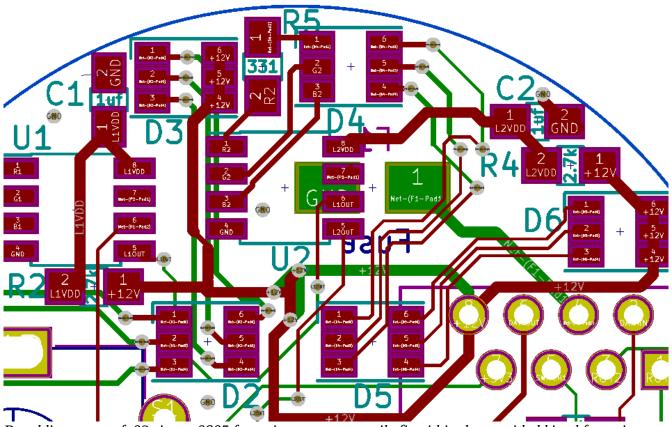
By adding a text of .02 size to 0805 footprints, you can easily fit within the provided kicad footprint. This makes soldering easier later. See here, labels such as 1uf, or 2.7k.
