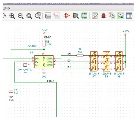
Adding net labels, makes line identification on layout easier. Here we have R3, G3, and B3, telling us that these leds are going to the input of the LED driver.
