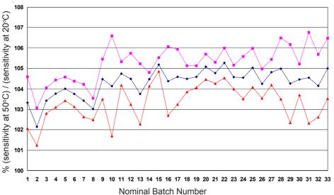
This plot of the mean and ±95% confidence intervals for 34 batches shows superior repeatability of the sensitivity dependence from batch to batch, giving confidence when setting temperature compensation in your gas detector.
