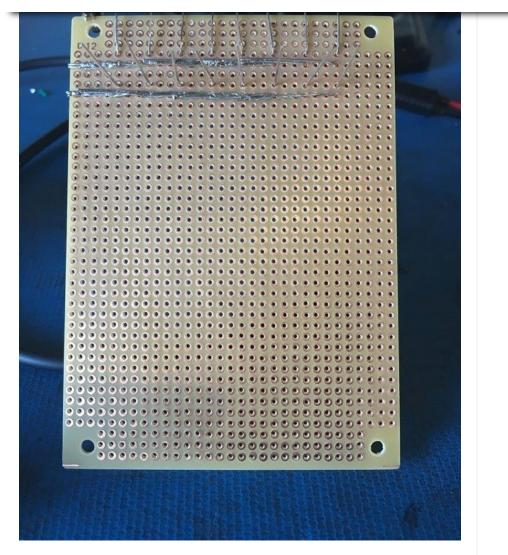
Once we've successfully soldered a row of cathodes, we can test their conductivity using a multimeter set to continuity mode.
