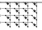
The difference between these two configurations determine how you would call on a specific LED. With common-row anode (left), the current sources (positive voltage) are attached to rows A – D. Currents sinks (negative voltage, ground) are attached to columns 1 – 4.
