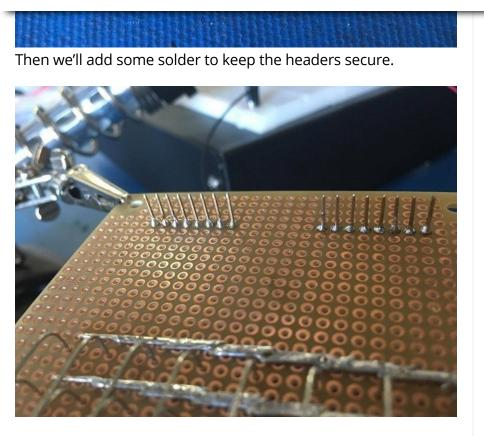
Now comes the (arguably) most difficult part of this build with regards to soldering skill.... connecting the pins to the rows and columns.
