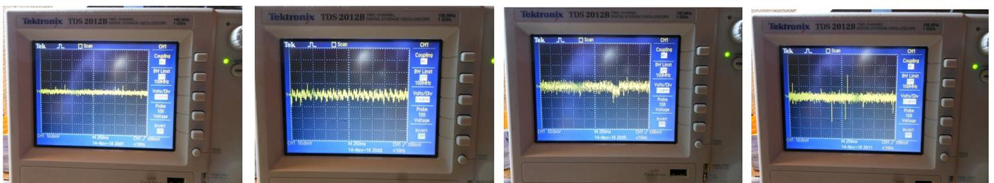
The HFS draws negligible power, in this application, <5mA. The ENC on the other hand... (ethernet or wifi are around 200mA each, 3.3v). I suspect capacity was the problem. Simply adding a capacitor to the HFS (I tried a 220uF name brand), did not resolve the issue. A worthy test would be an HFS with Arduino and no ENC. The usb power has limits that may be the culprit.
