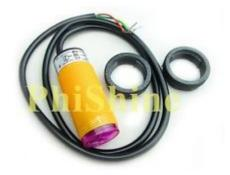
An example of a low cost photo electric sensor from ebay.
