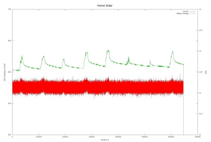
Data from 07-01 to 07-08-18 Note that a few cloudy days, cause the battery to discharge, (overall) with this setup. The current readings, do show a slight increase, though still in the noise. We need more panels.
