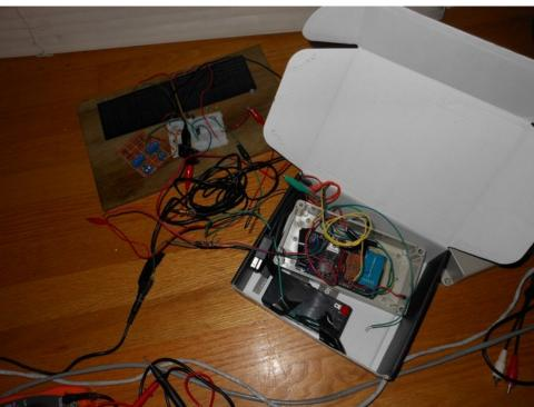
Windmill Data Logger was used with a 12V 1Ah battery. The Regulator used is a somewhat low power AP2204K-ADJTRG1, set to 13.7 or 13.8V (a float voltage for Lead Acid batteries I believe).
