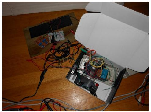
Windmill Data Logger was used with a 12V 1Ah battery. The Regulator used is a somewhat low power AP2204K-ADJTRG1, set to 13.7 or 13.8V (a float voltage for Lead Acid batteries I believe).
