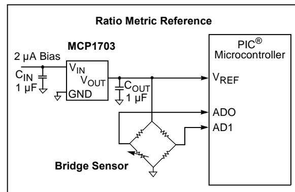
**FIGURE 6-2:** Using the MCP1703 as a Voltage Reference.
