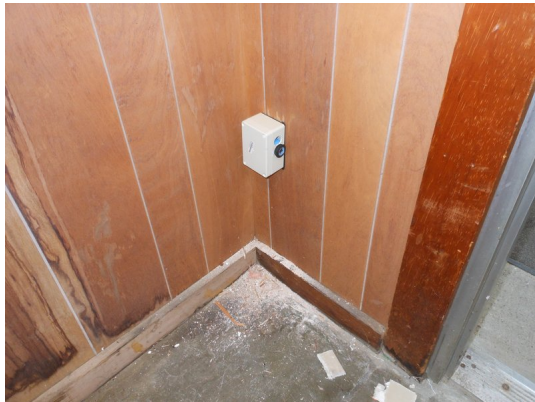
Figure 5: Part 1 of sensor. By mounting it on the right side of a project box, we can get a 90 degree angle.
