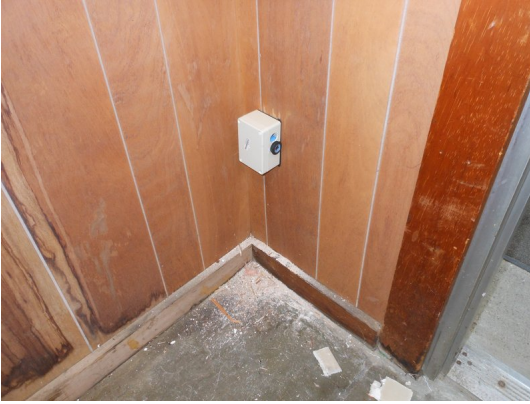
Figure 5: Part 1 of sensor. By mounting it on the right side of a project box, we can get a 90 degree angle.
