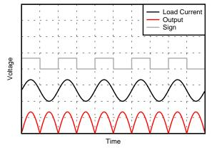
Figure 16. Bipolar Current Measurement Results (Arbitrary Scale)
