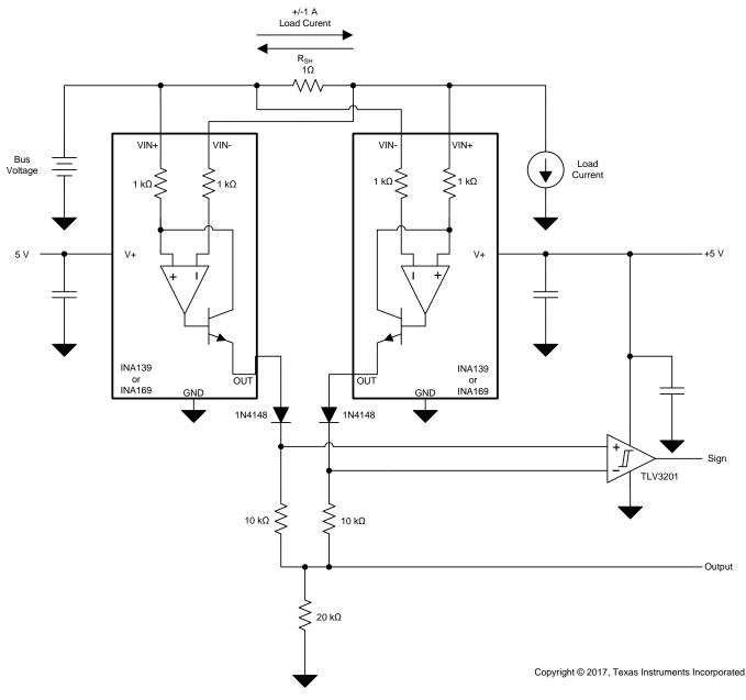
Figure 15. Bipolar Current Measurement
