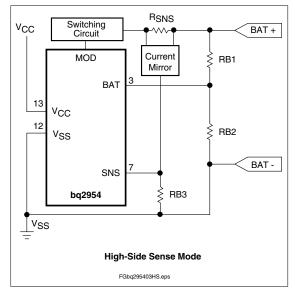
Figure 7. Configuring the Battery Divider (High-Side Sense)
