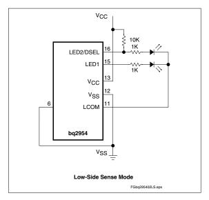
Figure 4. Configured Display Mode (Low-Side Sense)
