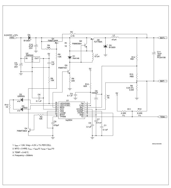
Figure 3. High-Efficiency Li-lon Charger for 1-4 Cells
