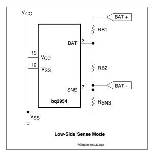
Figure 6. Configuring the Battery Divider (Low-Side Sense)
