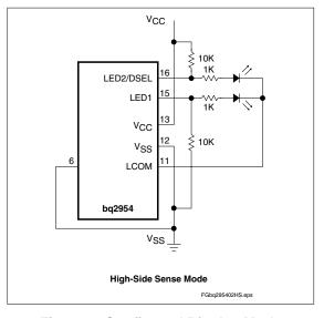
Figure 5. Configured Display Mode (High-Side Sense)
