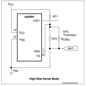
Figure 9. High-Side Temperature Sensing
