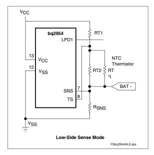
Figure 8. Low-Side Temperature Sensing
