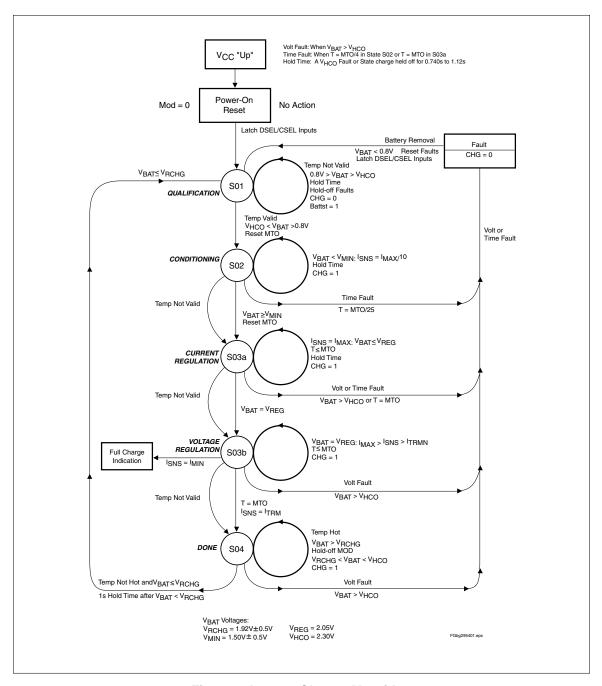
Figure 2. bq2954 Charge Algorithm
