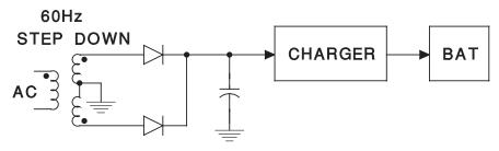
Figure 5. Isolated Off Line Charger
