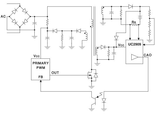
Figure 4. Off Line Charger With Primary Side PWM
