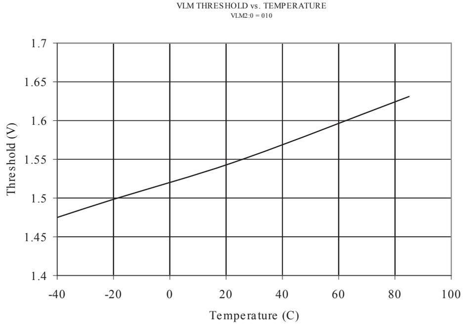
**Figure 18-44. VLM2 Threshold of V<sub>CC</sub> Level Monitor**
