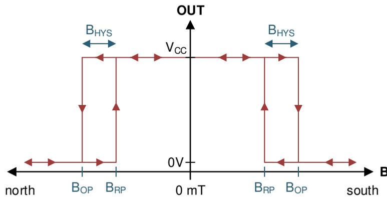
Figure 16. Omnipolar Functionality
