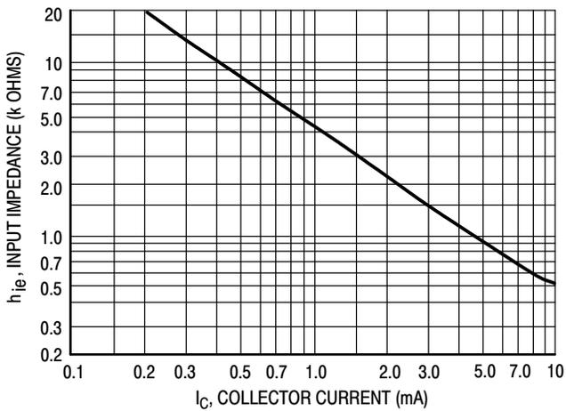
Figure 11. Input Impedance
