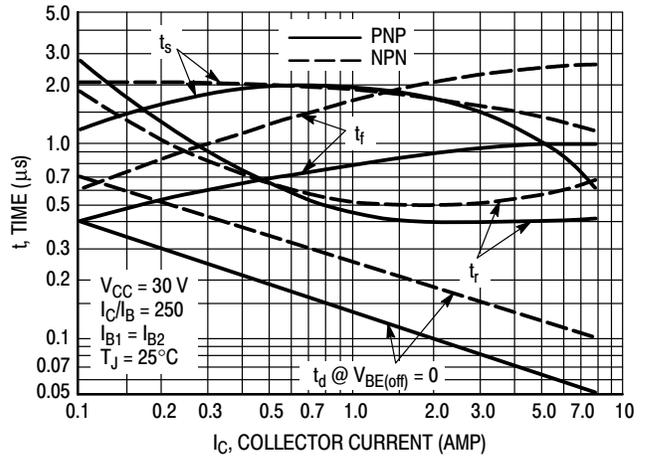
Figure 4. Switching Times
