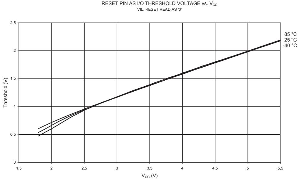
**Figure 18-32. Reset Input Hysteresis vs.  $V_{CC}$  (Reset Pin Used as I/O)**
