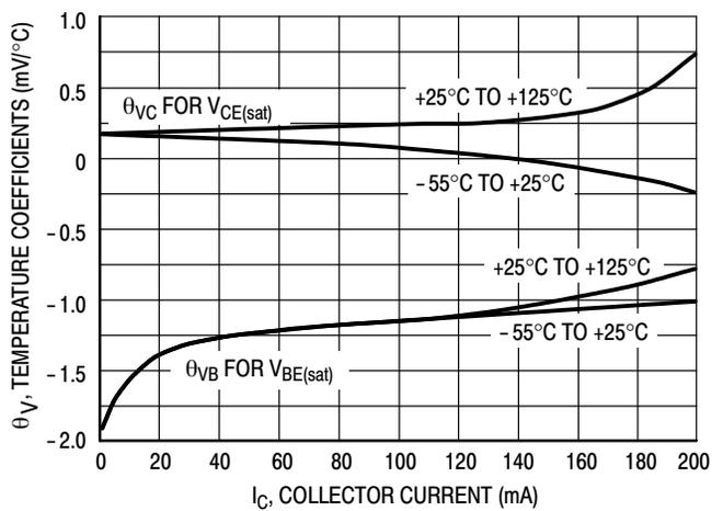
Figure 16. Temperature Coefficients
