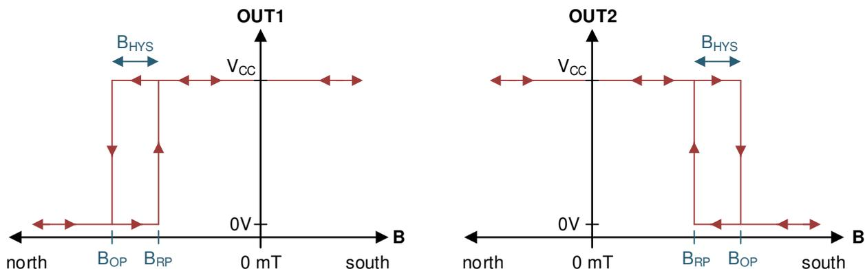
Figure 17. Unipolar Functionality
