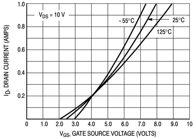
Figure 2. Transfer Characteristics
