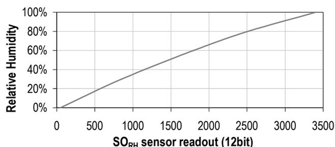
**Figure 18:** Conversion from SO<sub>RH</sub> to relative humidity
