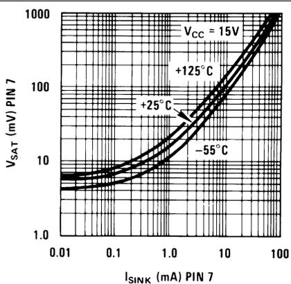
Figure 9. Discharge Transistor (Pin 7) Voltage vs. Sink Current
