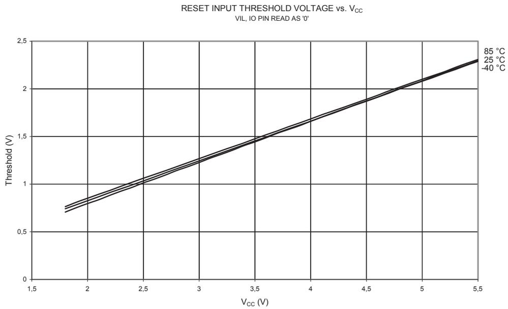
Figure 18-35. Reset Pin, Input Hysteresis vs.  $V_{CC}$
