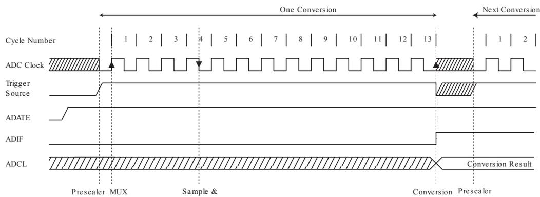
In Free Running mode, a new conversion will be started immediately after the conversion completes, while ADCRSA.ADSC remains high. See also the ADC Conversion Time table below.
