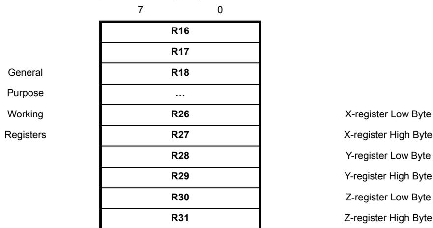
**Note:** A typical implementation of the AVR register file includes 32 general purpose registers but ATtiny4/5/9/10 implement only 16 registers. For reasons of compatibility the registers are numbered R16...R31, not R0...R15.
