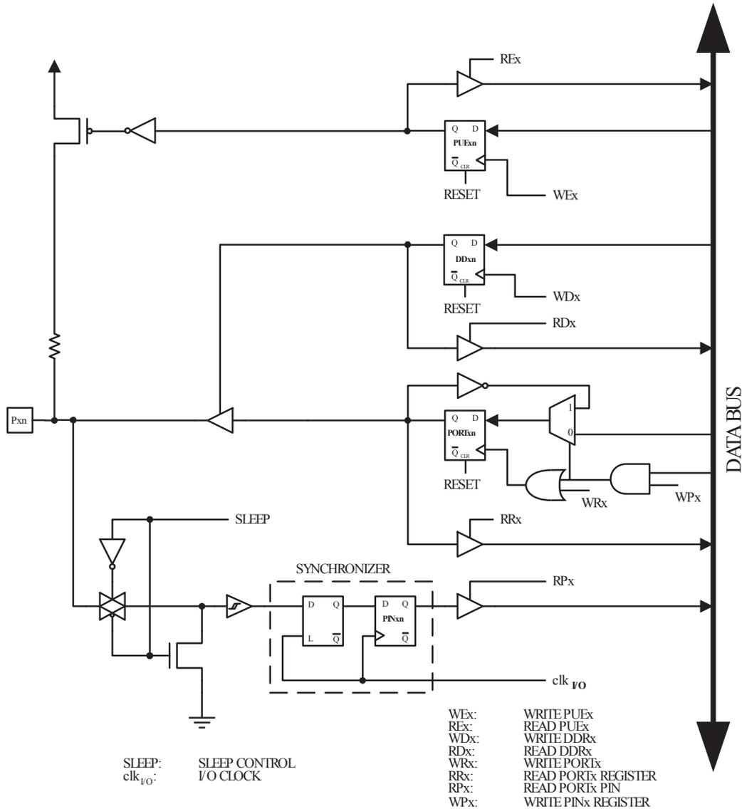
**Note:** WEx, WRx, WPx, WDx, REx, RRx, RPx, and RDx are common to all pins within the same port. clk<sub>I/O</sub>, SLEEP are common to all ports.
