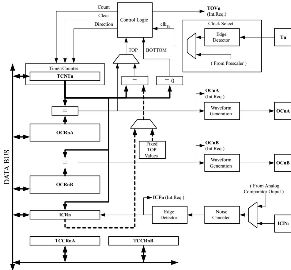
**Note:** The “n” in the register and bit names indicates the device number (n = 0 for Timer/Counter 0)
