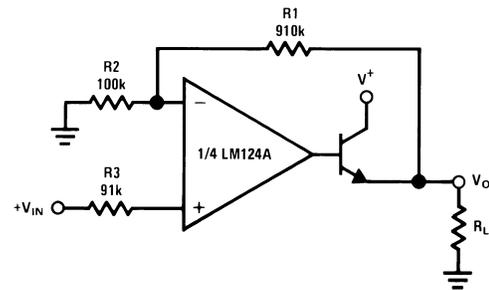
Where:  $V_0 = 0 V_{DC}$  for  $V_{IN} = 0 V_{DC}$
