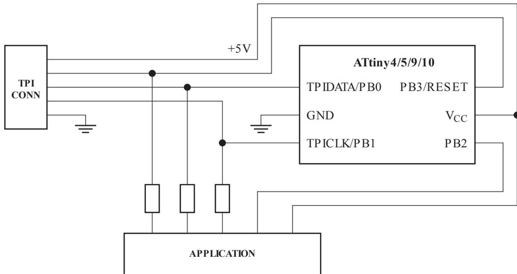
NVM can be programmed at 5V, only. In some designs it may be necessary to protect components that can not tolerate 5V with, for example, series resistors.
