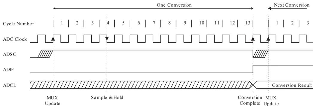
When Auto Triggering is used, the prescaler is reset when the trigger event occurs, as the next figure. This assures a fixed delay from the trigger event to the start of conversion. In this mode, the sample-and-
