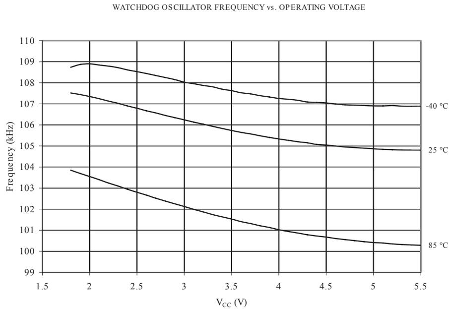
Figure 18-38. Watchdog Oscillator Frequency vs. Temperature
