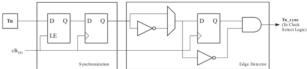
**Note:** The “n” indicates the device number ( $n = 0$  for Timer/Counter 0)
