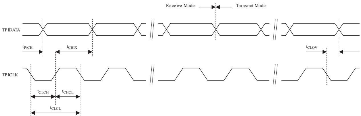
**Table 17-9. Serial Programming Characteristics,  $T_A = -40^{\circ}\text{C}$  to  $85^{\circ}\text{C}$ ,  $V_{CC} = 5\text{V} \pm 5\%$  (Unless Otherwise Noted)**
