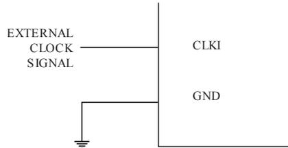
When applying an external clock, it is required to avoid sudden changes in the applied clock frequency to ensure stable operation of the MCU. A variation in frequency of more than 2% from one clock cycle to the next can lead to unpredictable behavior. It is required to ensure that the MCU is kept in Reset during the changes.
