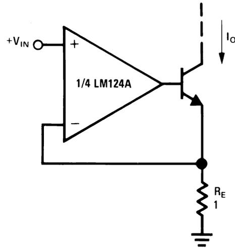
$$I_O = 1 \text{ amp/volt } V_{IN} \text{ (Increase } R_E \text{ for } I_O \text{ small)}$$
