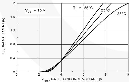
Figure 5. Transfer Characteristics
