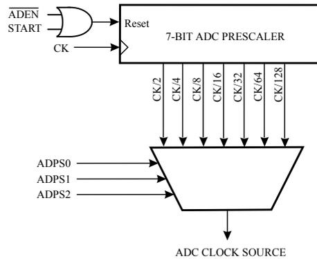
When initiating a single ended conversion by writing a '1' to the ADC Start Conversion bit (ADCSRA.ADSC), the conversion starts at the following rising edge of the ADC clock cycle.
