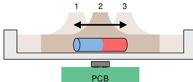
Figure 25. Three-Position Slider Switch With Embedded Magnet
