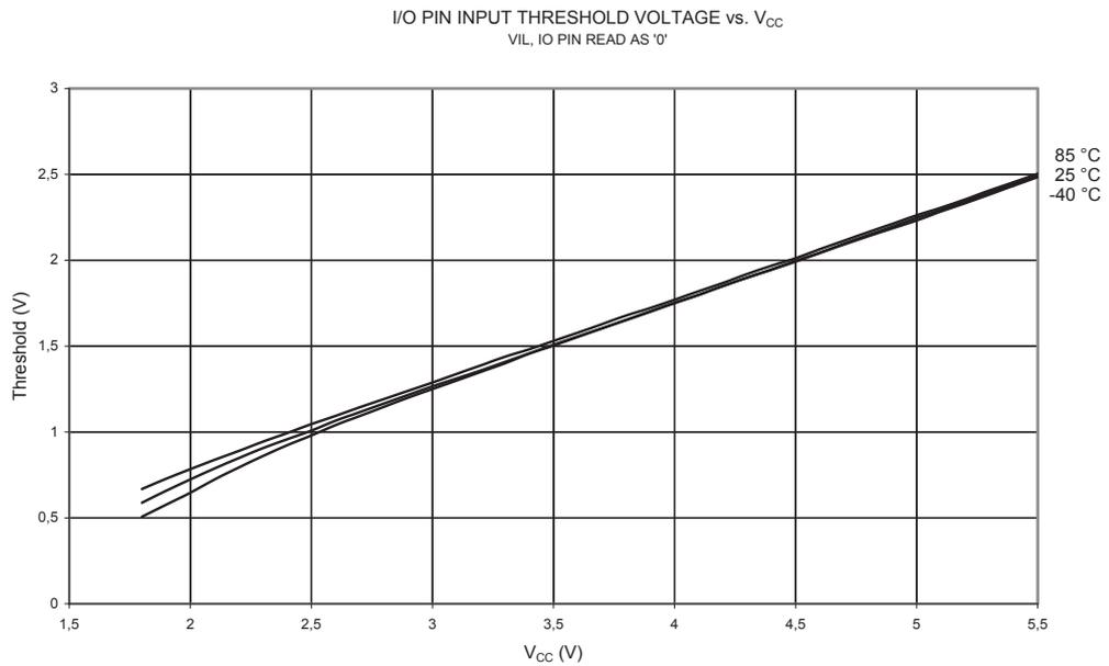
**Figure 18-29. I/O Pin Input Hysteresis vs.  $V_{CC}$**
