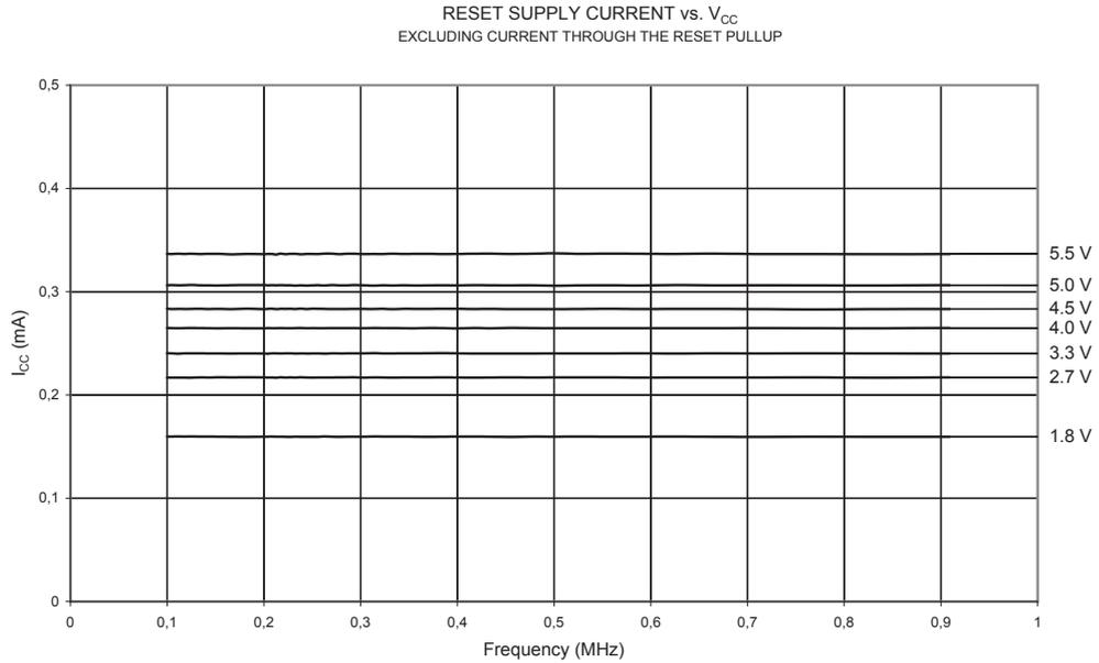
**Note:** The default clock source for the device is always the internal 8 MHz oscillator. Hence, current consumption in reset remains unaffected by external clock signals.
