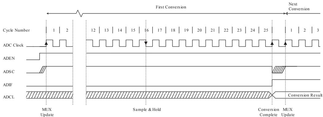
The actual sample-and-hold takes place 3 ADC clock cycles after the start of a normal conversion and 16 ADC clock cycles after the start of an first conversion. When a conversion is complete, the result is written to the ADC Data Registers (ADCL), and the ADC Interrupt Flag (ADCSRA.ADIF) is set. In Single Conversion mode, ADCSRA.ADSC is cleared simultaneously. The software may then set ADCSRA.ADSC again, and a new conversion will be initiated on the first rising ADC clock edge.
