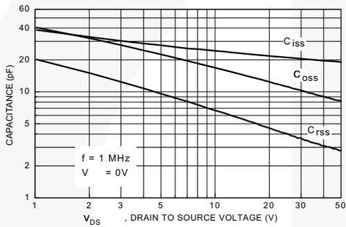
**Figure 9. Capacitance Characteristics**
