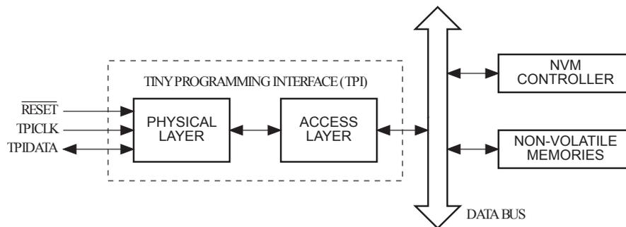
Programming is done via the physical interface. This is a 3-pin interface, which uses the  $\overline{\text{RESET}}$  pin as enable, the TPICLK pin as the clock input, and the TPIDATA pin as data input and output. NVM can be programmed at 5V, only.
