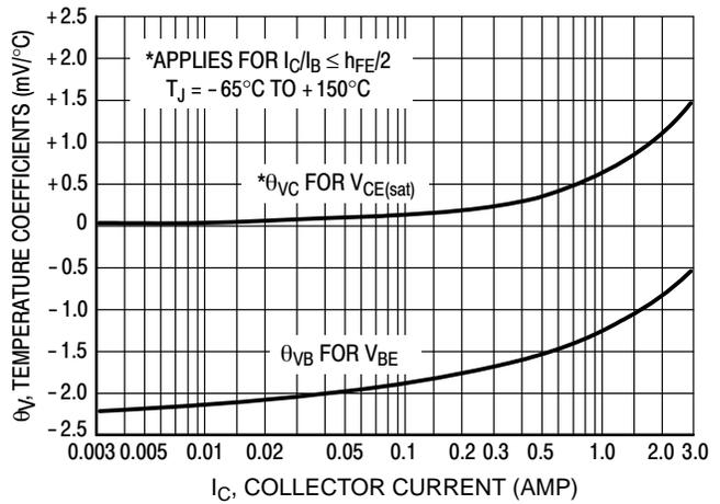
Figure 11. Temperature Coefficients
