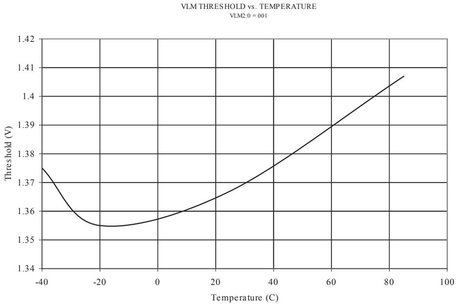
**Figure 18-43. VLM1H Threshold of V<sub>CC</sub> Level Monitor**
