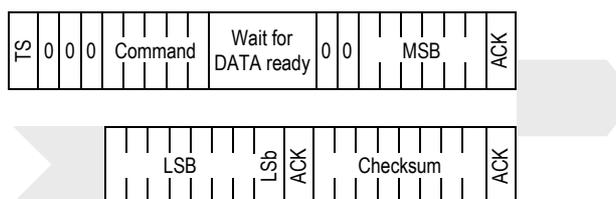
Figure 16: Overview of Measurement Sequence. TS = Transmission Start, MSB = Most Significant Bit, LSB = Last Significant Byte, LSb = Last Significant Bit.
