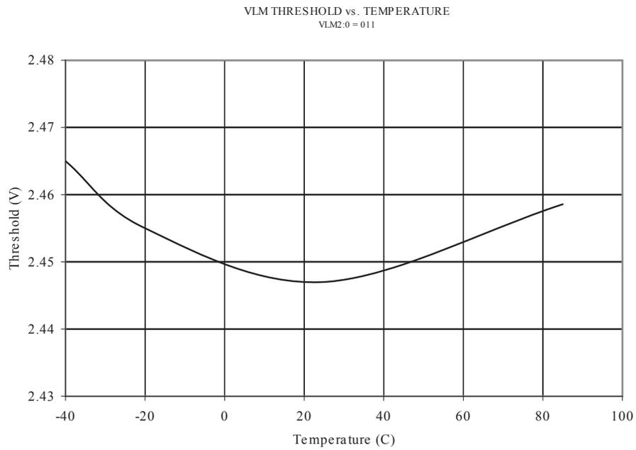
Figure 18-45. VLM3 Threshold of V<sub>CC</sub> Level Monitorr2
