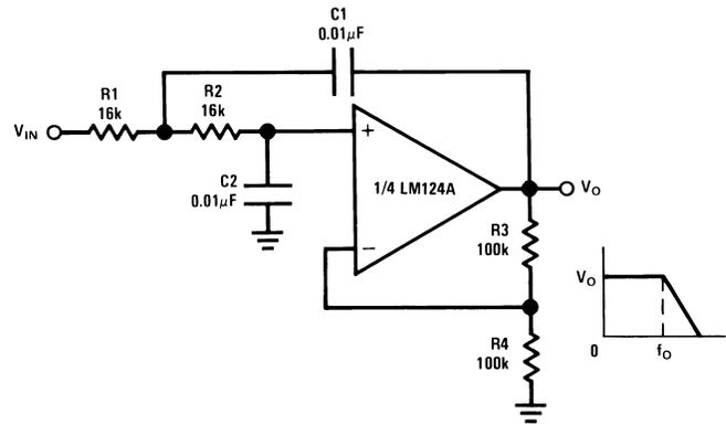
Figure 35. DC Coupled Low-Pass RC Active Filter
