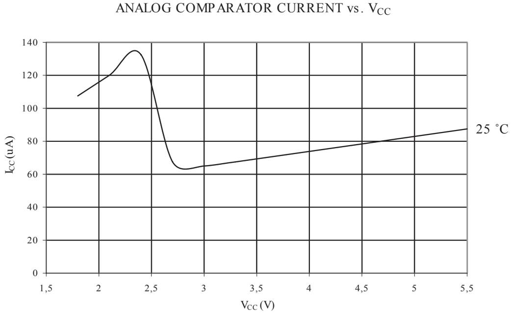
Figure 18-48. V<sub>CC</sub> Level Monitor Current vs. V<sub>CC</sub>
