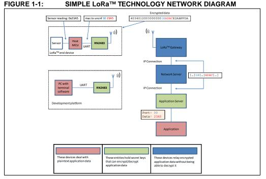
The flow of data can be followed as it gets generated by an end device and transported on the network.
