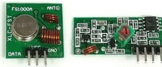
Figure 1: simple rx tx on 433mhz
