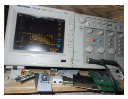
Figure 2: With a \_delay\_ms, there is no ramping up. But, the delay had to be a minimum, otherwise some ramping did occur. It's very slow, but usable for things without a lot of data to transmit.
