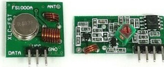
Figure 2: simple rx tx on 433mhz
