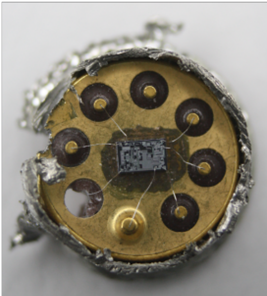
Inside a 741 op amp, showing the die. This is a TO-99 metal can package, with the top sawed off
