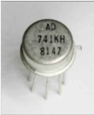
The 741 op amp, packaged in a TO-99 metal can.
