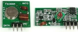
Figure 4: simple rx tx on 433mhz
