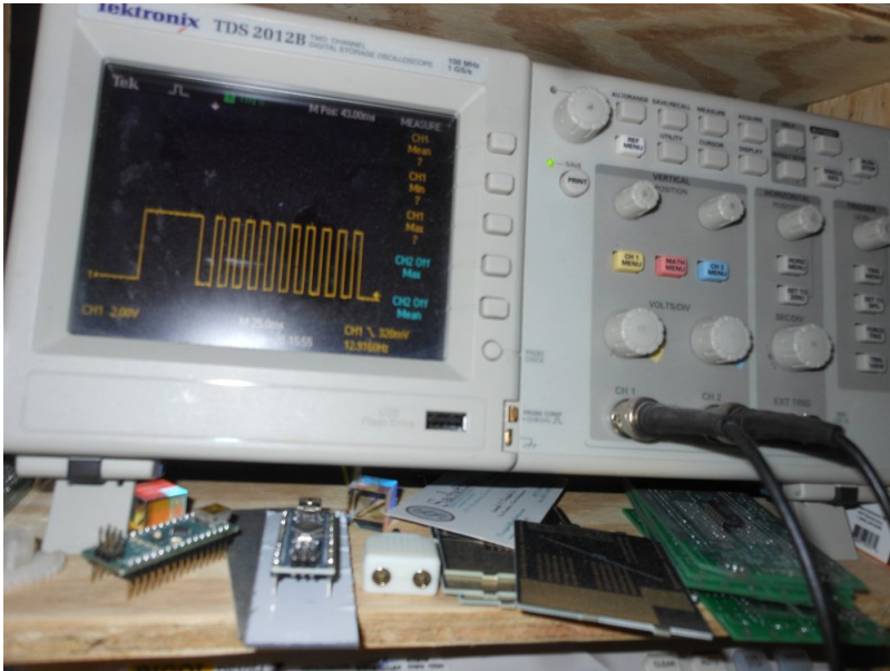
Figure 5: With a _delay_ms , there is no ramping up. But, the delay had to be a minimum, otherwise some ramping did occur. It's very slow, but usable for things without a lot of data to transmit.
