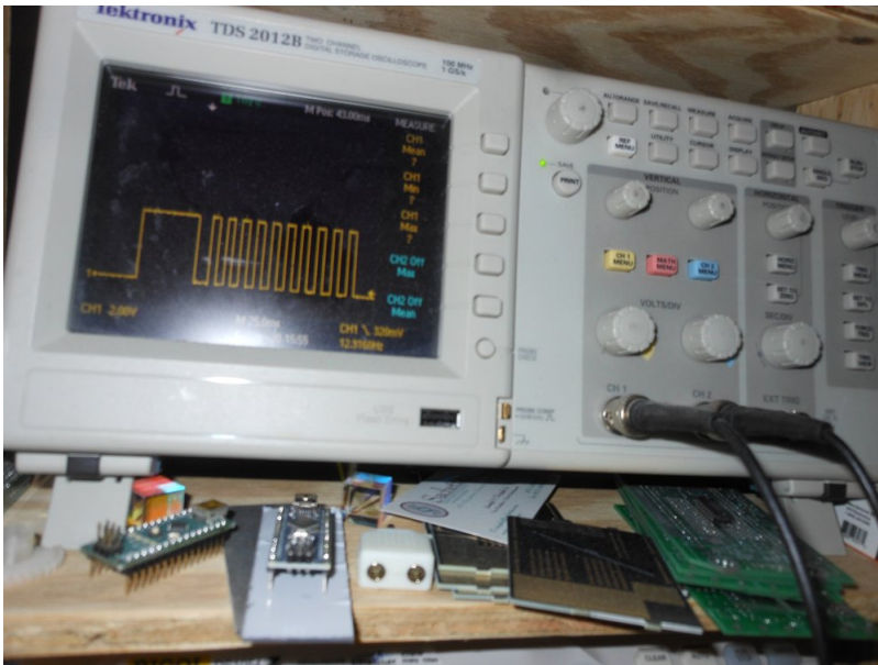
Figure 4: With a _delay_ms , there is no ramping up. But, the delay had to be a minimum, otherwise some ramping did occur. It's very slow, but usable for things without a lot of data to transmit.
