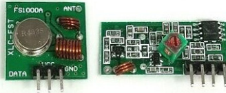
Figure 3: simple rx tx on 433mhz
