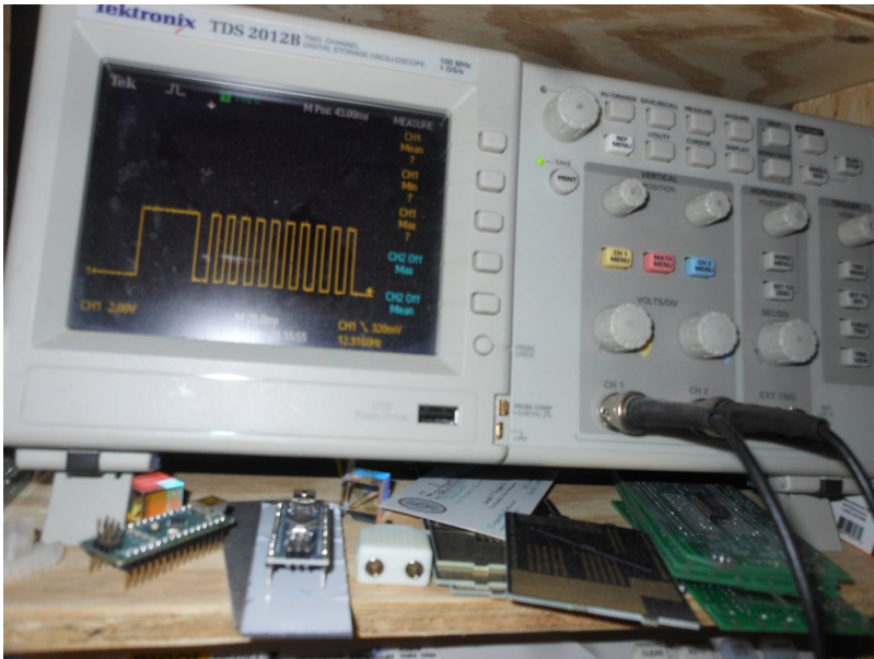
Figure 2: With a _delay_ms , there is no ramping up. But, the delay had to be a minimum, otherwise some ramping did occur. It's very slow, but usable for things without a lot of data to transmit.
