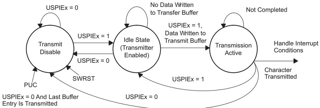
Figure 19-4. Master Transmit Enable State Diagram
