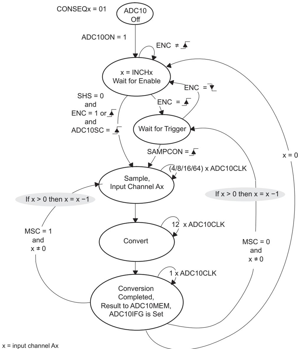
Figure 22-6. Sequence-of-Channels Mode
