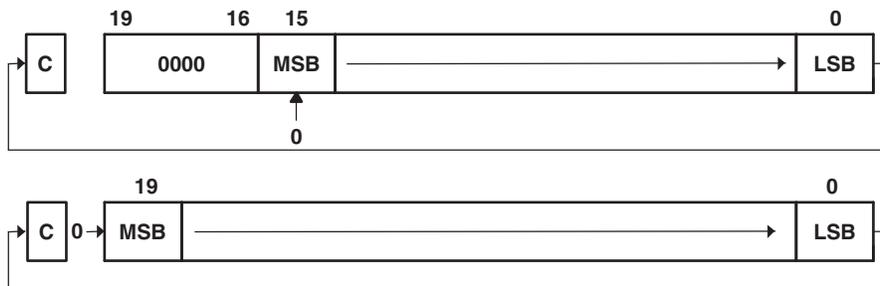
Figure 4-52. Rotate Right Unsigned RRUM[.W] and RRUM.A
