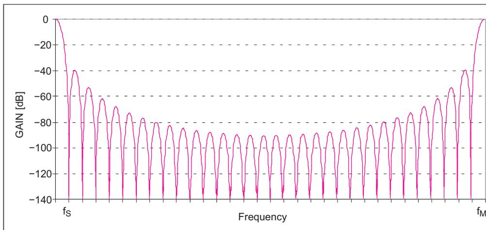
**Figure 26-3. Comb Filter Frequency Response With OSR = 32**
