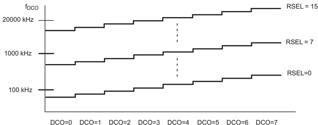
Figure 5-6. Typical DCOx Range and RSELx Steps
