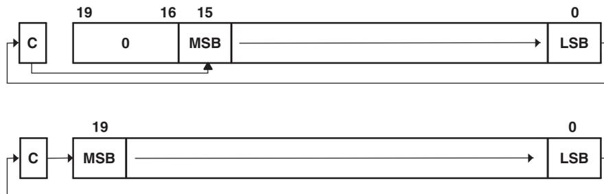
**Figure 4-49. Rotate Right Through Carry RRCM.[W] and RRCM.A**
