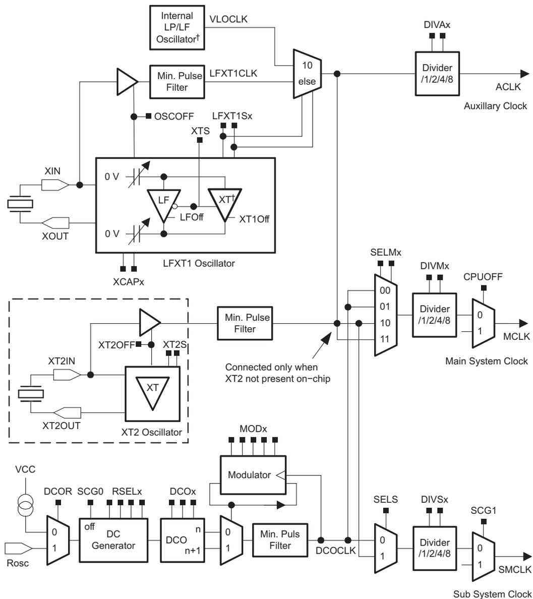
**Figure 5-1. Basic Clock Module+ Block Diagram – MSP430F2xx**
