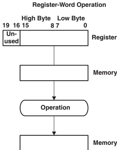
Figure 4-11. Register-Word Operation
