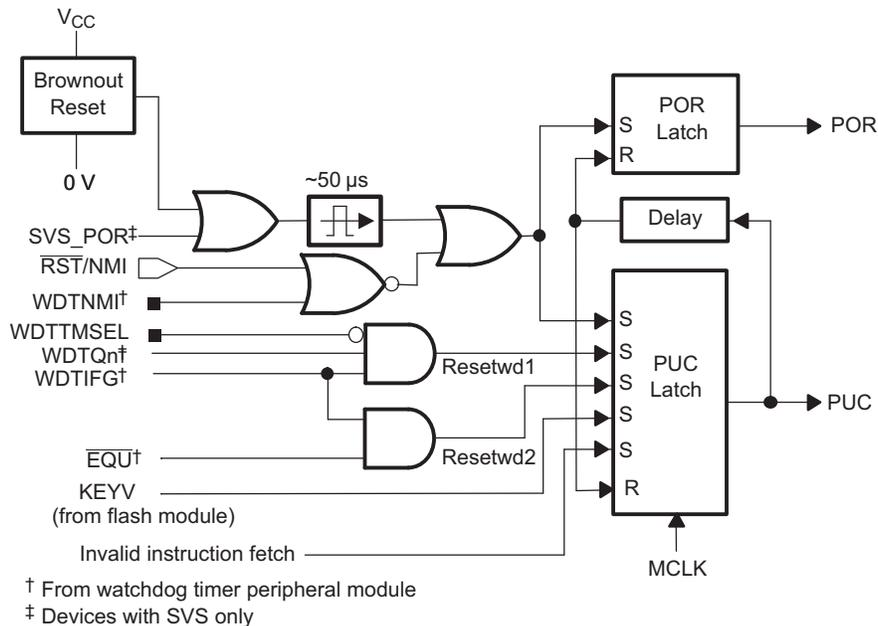
**Figure 2-1. Power-On Reset and Power-Up Clear Schematic**
