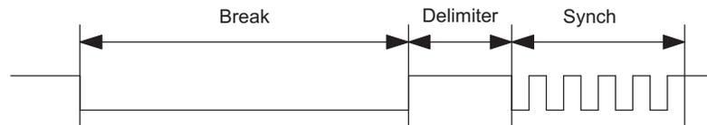
**Figure 15-5. Auto Baud Rate Detection - Break/Synch Sequence**
