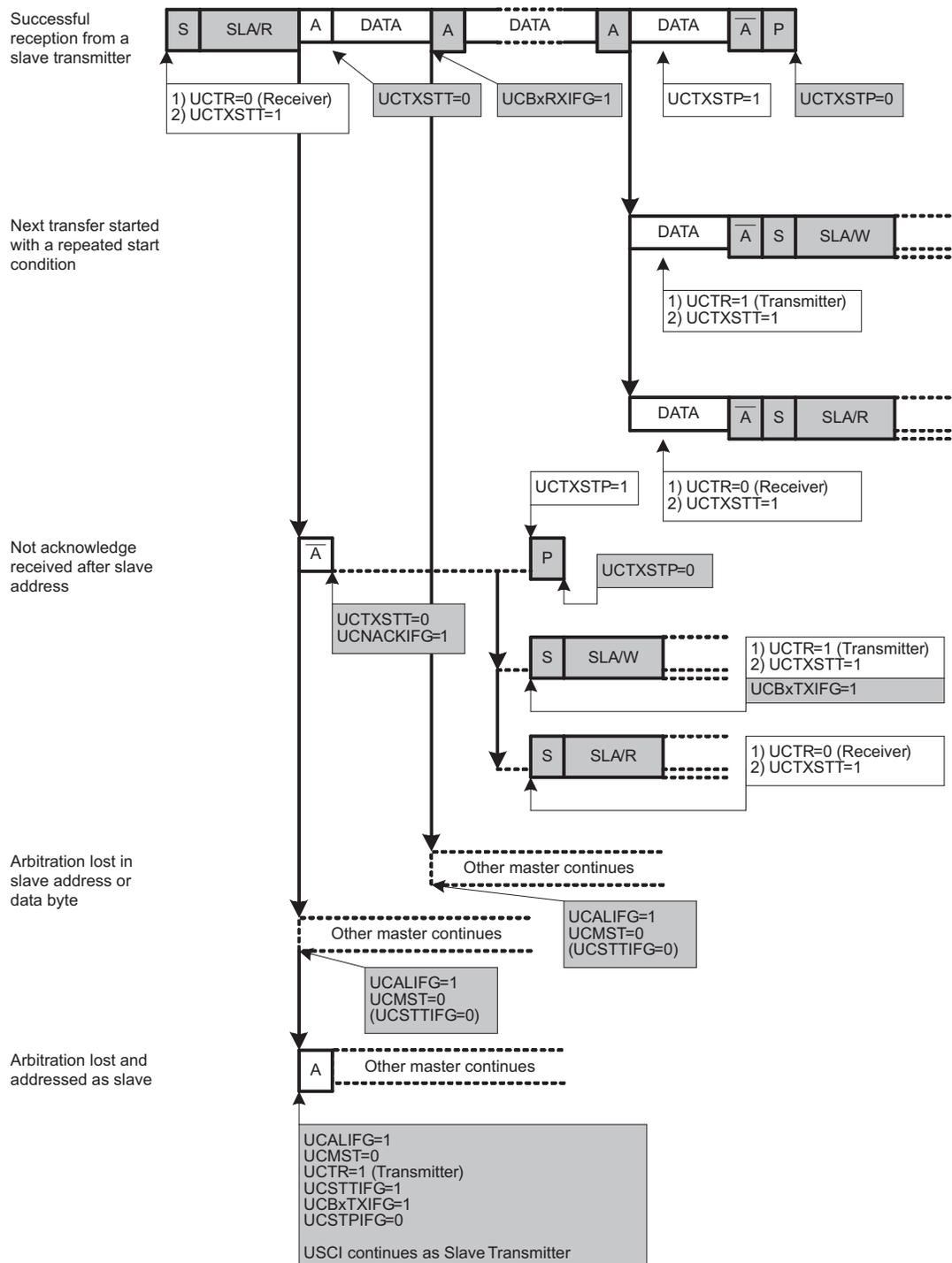
Figure 17-13. I<sup>2</sup>C Master Receiver Mode
