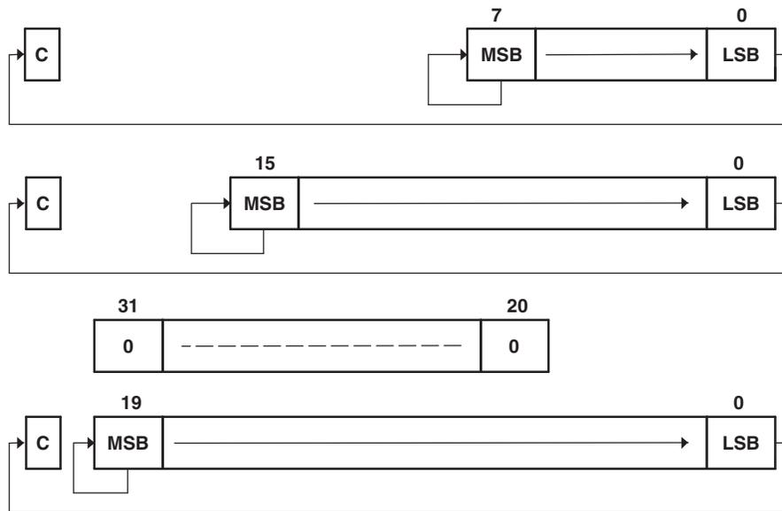
Figure 4-48. Rotate Right Arithmetically RRAX(.B,.A) – Non-Register Mode
