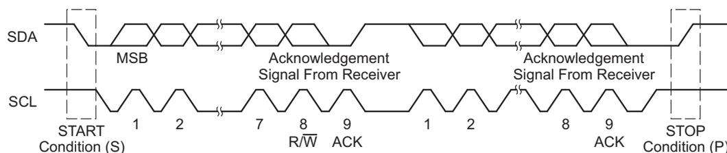
**Figure 17-3. I<sup>2</sup>C Module Data Transfer**
