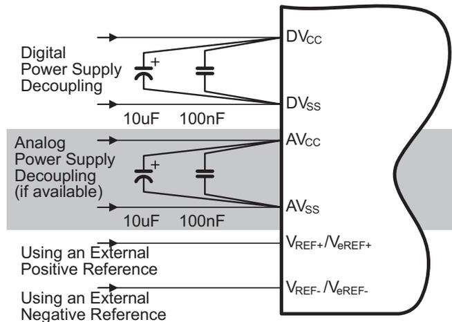
Figure 22-15. ADC10 Grounding and Noise Considerations (External  $V_{REF}$ )
