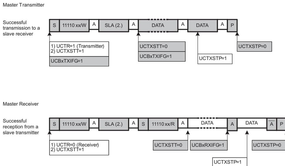
Figure 17-14. I<sup>2</sup>C Master 10-bit Addressing Mode
