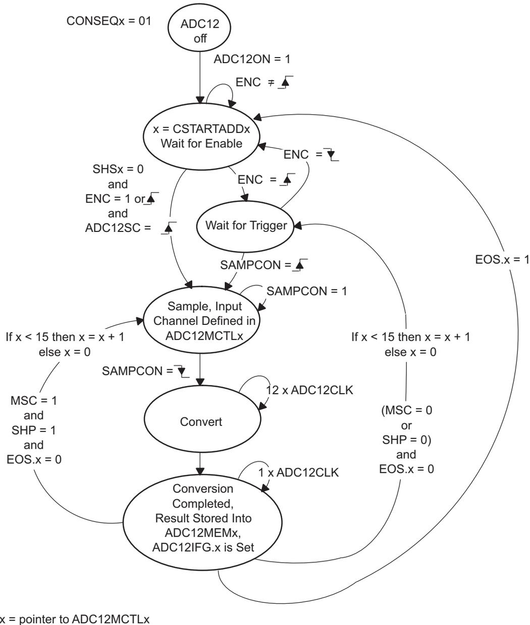
Figure 23-7. Sequence-of-Channels Mode
