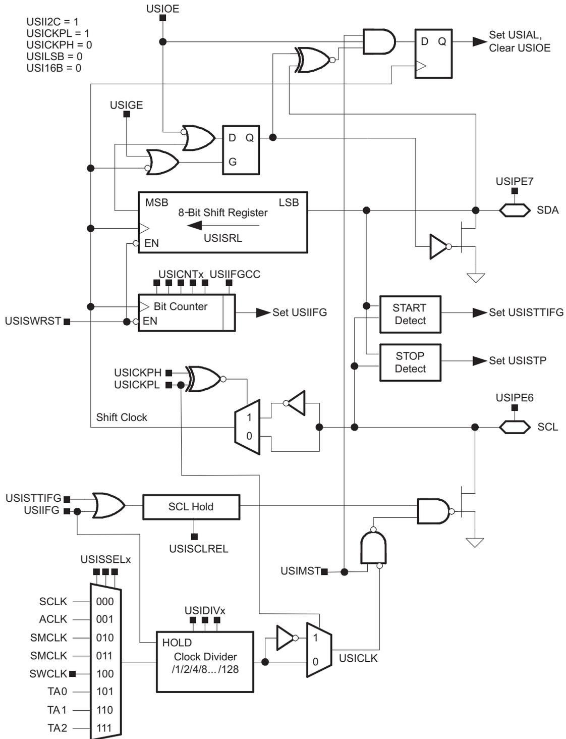
Figure 14-2. USI Block Diagram: I<sup>2</sup>C Mode
