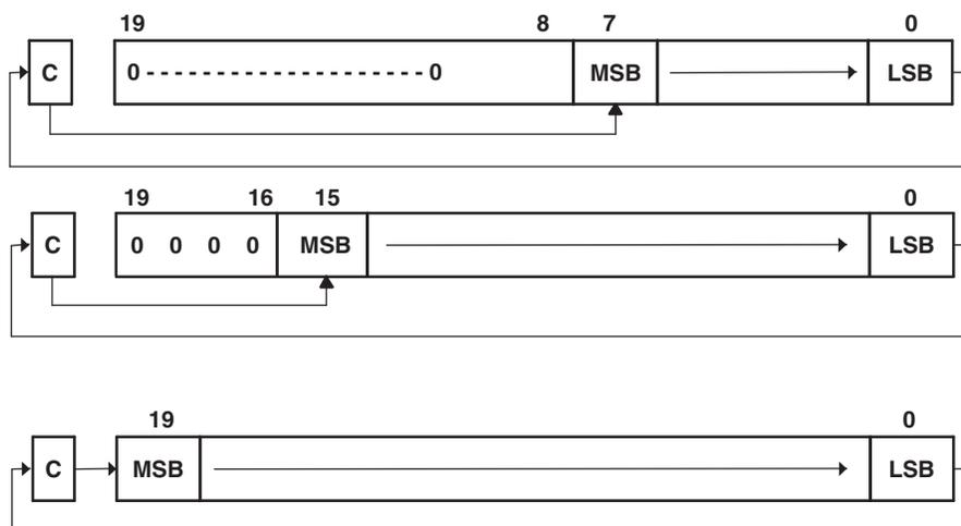
Figure 4-50. Rotate Right Through Carry RRCX(.B,.A) – Register Mode
