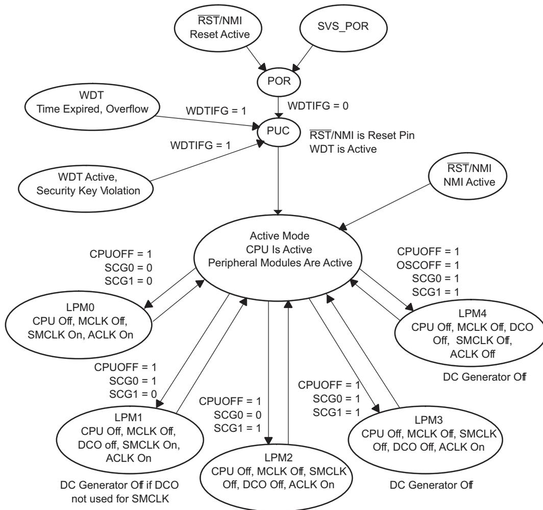
Figure 2-9. Operating Modes For Basic Clock System
