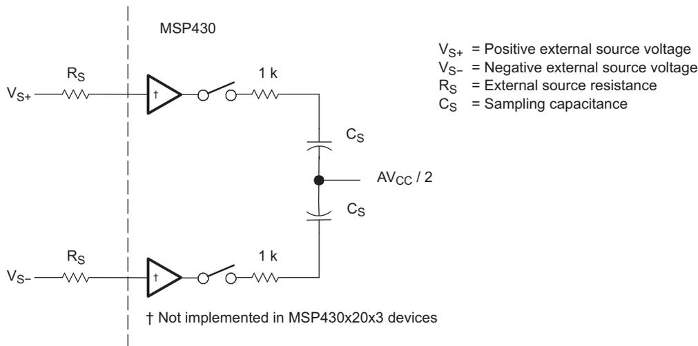
**Figure 26-2. Analog Input Equivalent Circuit**
