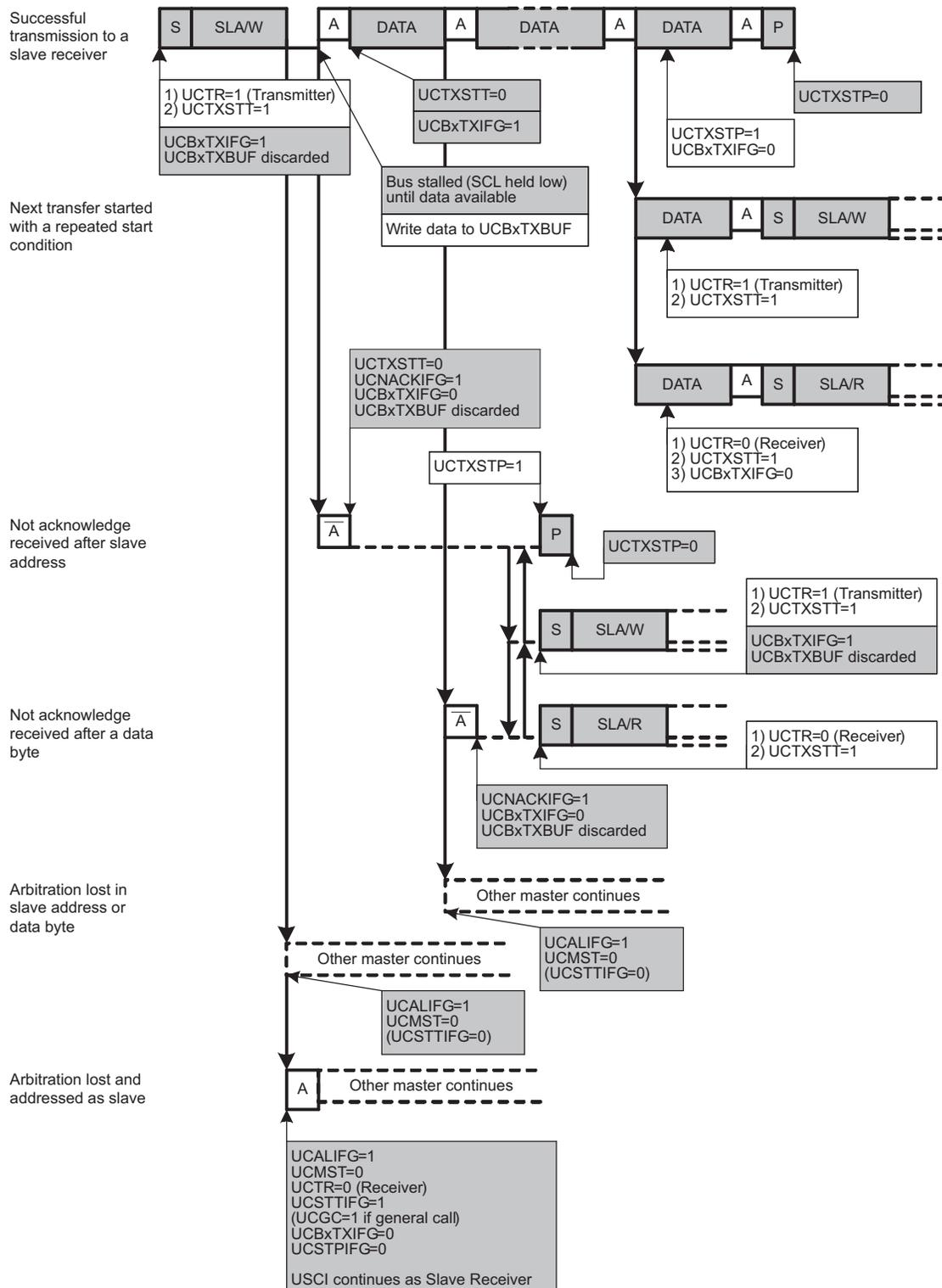
Figure 17-12. I<sup>2</sup>C Master Transmitter Mode
