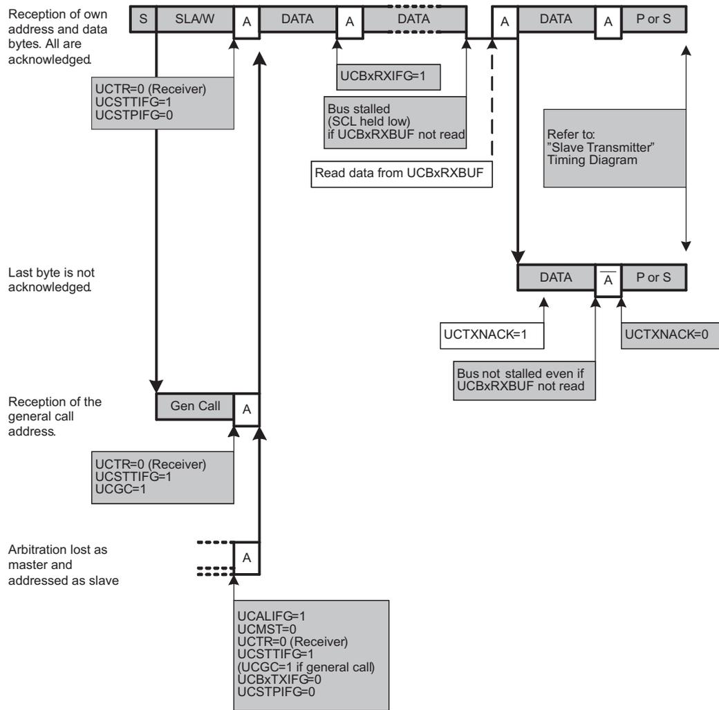
Figure 17-10. I<sup>2</sup>C Slave Receiver Mode
