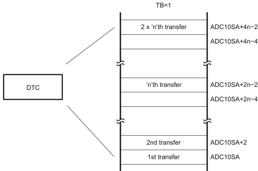
Figure 22-11. Two-Block Transfer
