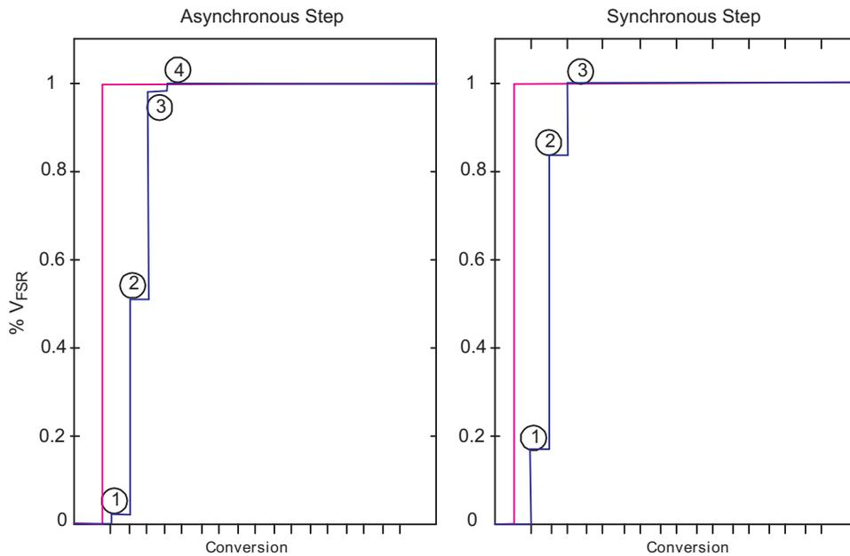
Figure 27-4. Digital Filter Step Response and Conversion Points
