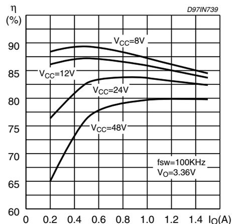
Figure 18. Efficiency vs. output current.
