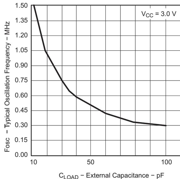
**Figure 8-2. Typical Pin-Oscillation Frequency**
