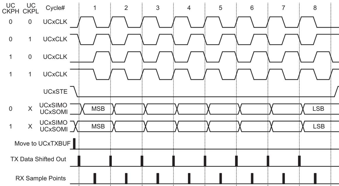
**Figure 16-4. USCI SPI Timing with UCMSB = 1**
