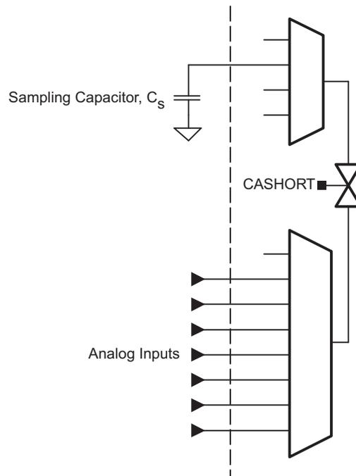
**Figure 21-2. Comparator\_A+ Sample-And-Hold**
