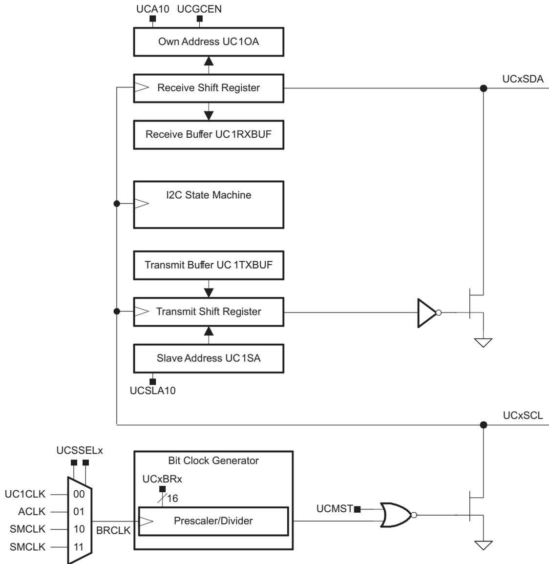
Figure 17-1. USCI Block Diagram: I<sup>2</sup>C Mode
