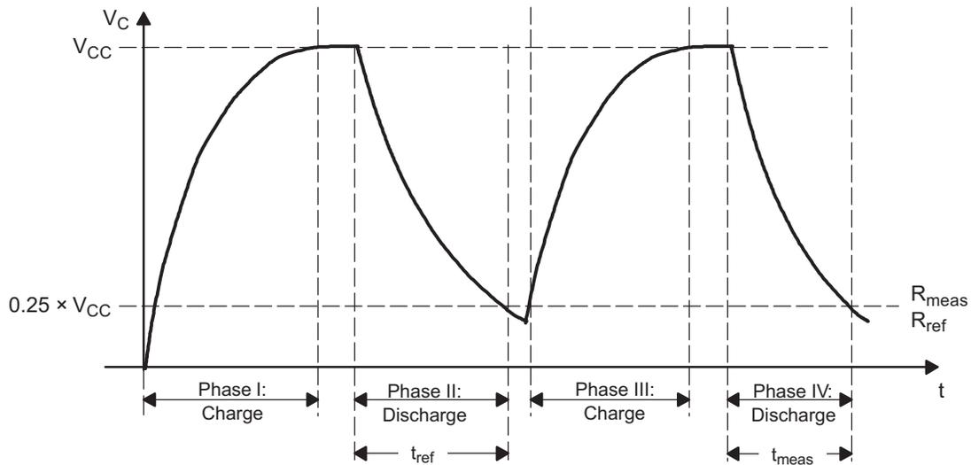
**Figure 21-7. Timing for Temperature Measurement Systems**
