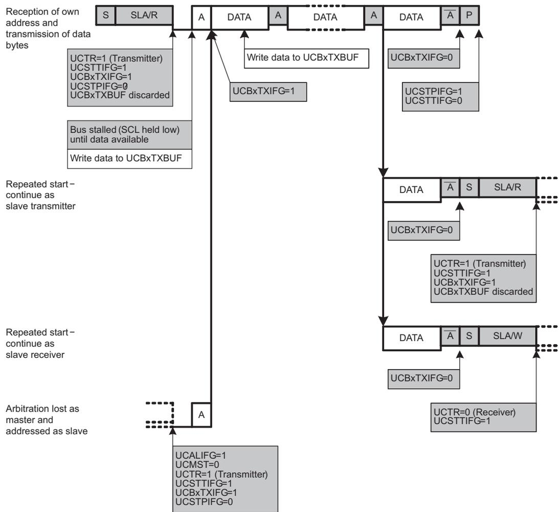
Figure 17-9. I<sup>2</sup>C Slave Transmitter Mode
