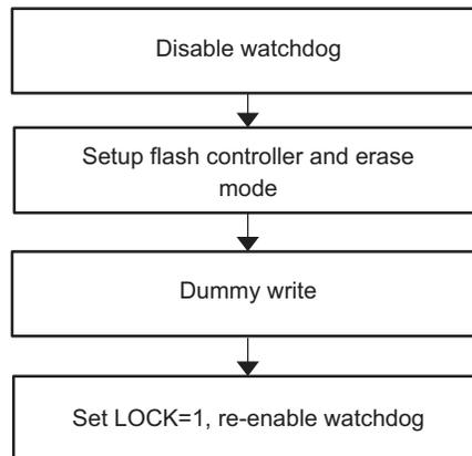
**Figure 7-5. Erase Cycle from Within Flash Memory**
