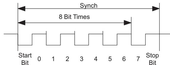
**Figure 15-6. Auto Baud Rate Detection - Synch Field**
