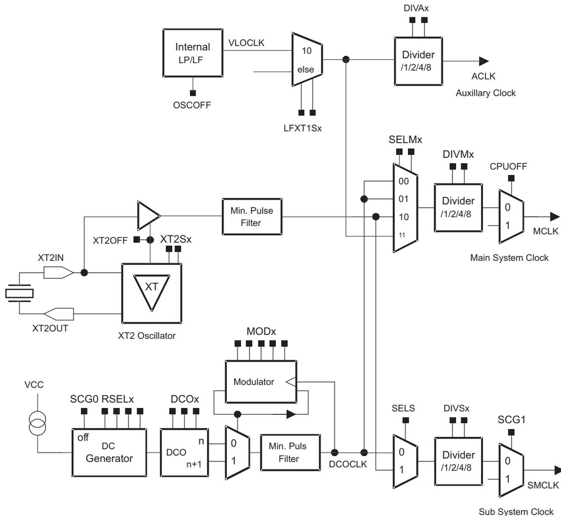
Figure 5-2. Basic Clock Module+ Block Diagram - MSP430AFE2xx
