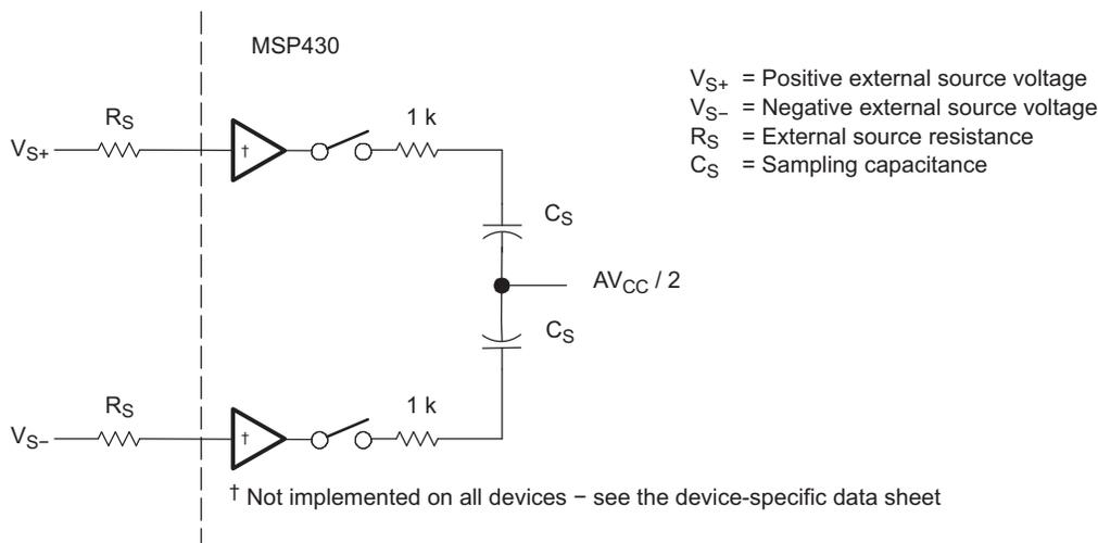
**Figure 27-2. Analog Input Equivalent Circuit**
