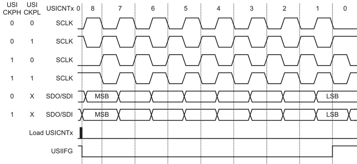
**Figure 14-3. SPI Timing**
