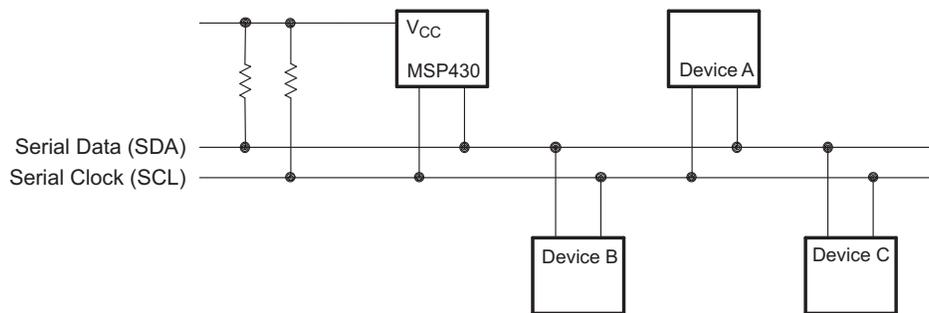
**Figure 17-2. I<sup>2</sup>C Bus Connection Diagram**
