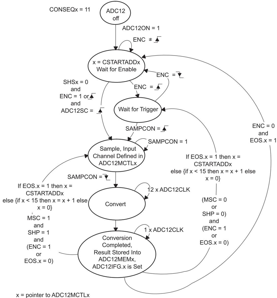
Figure 23-9. Repeat-Sequence-of-Channels Mode
