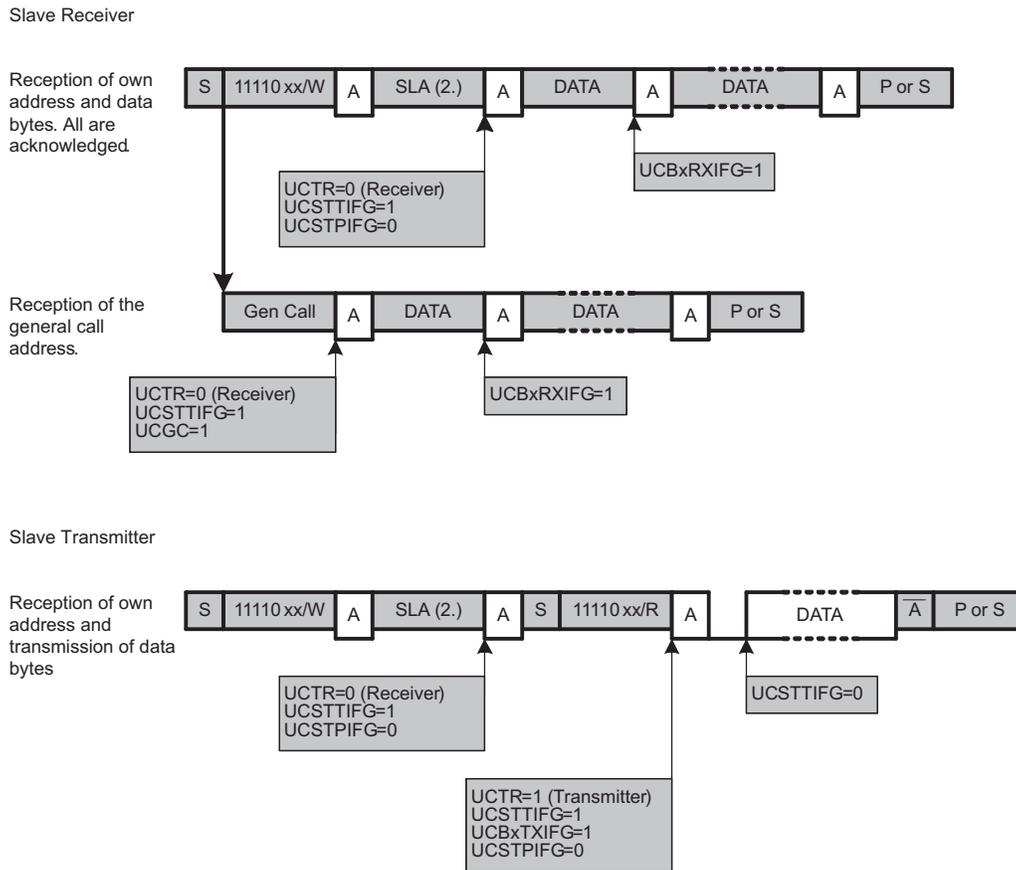
Figure 17-11. I<sup>2</sup>C Slave 10-bit Addressing Mode
