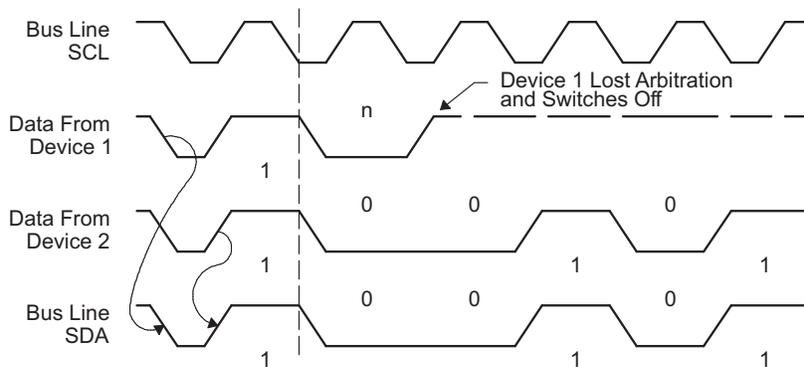
Figure 17-15. Arbitration Procedure Between Two Master Transmitters
