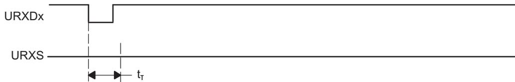
Figure 18-12. Glitch Suppression, USART Receive Not Started
