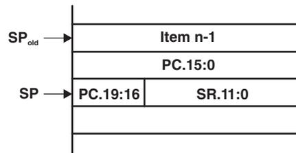
**Figure 4-2. PC Storage on the Stack for Interrupts**
