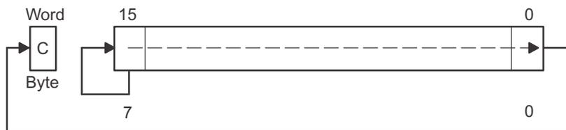
**Figure 3-17. Destination Operand – Arithmetic Right Shift**
