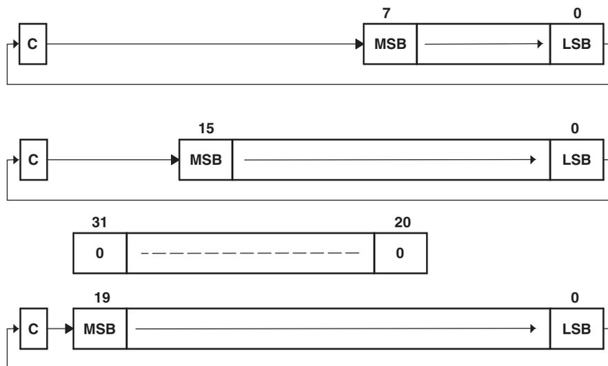
Figure 4-51. Rotate Right Through Carry RRCX(.B,.A) – Non-Register Mode
