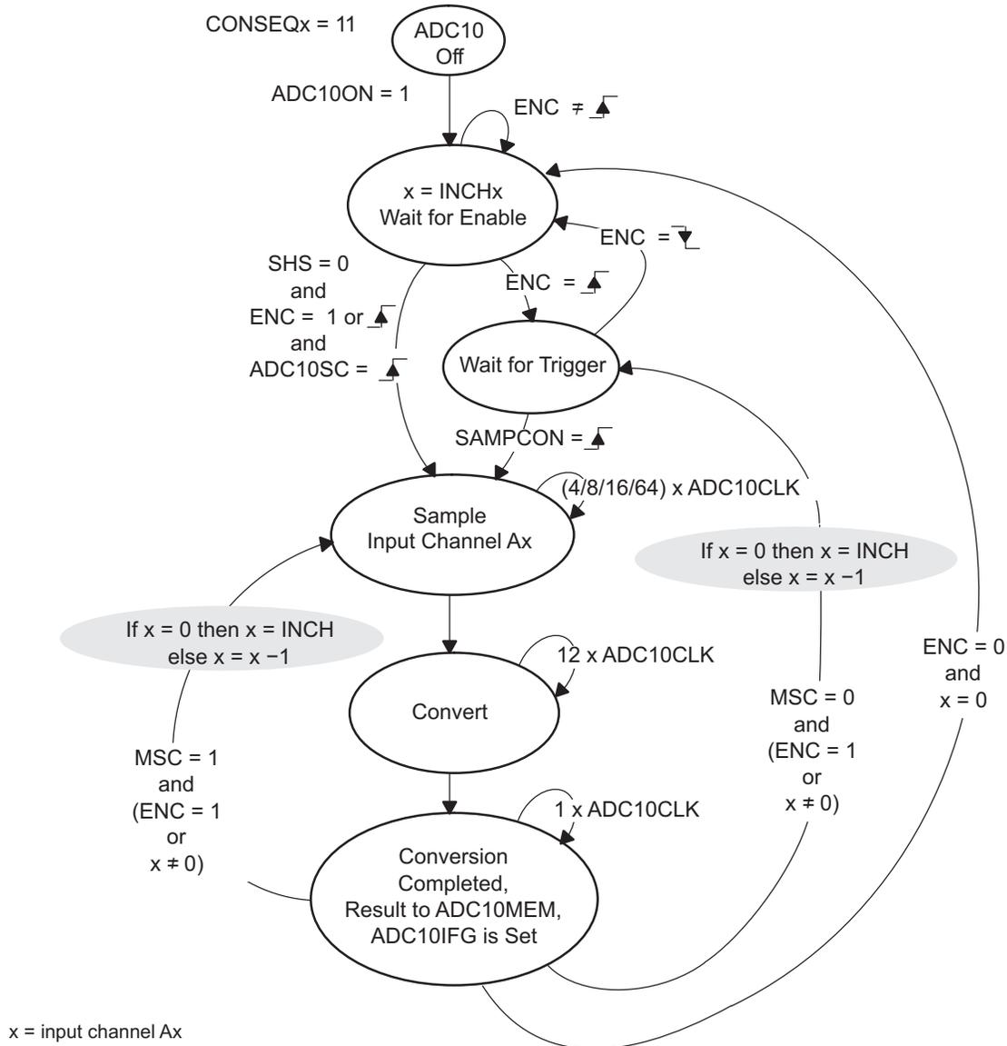
Figure 22-8. Repeat-Sequence-of-Channels Mode
