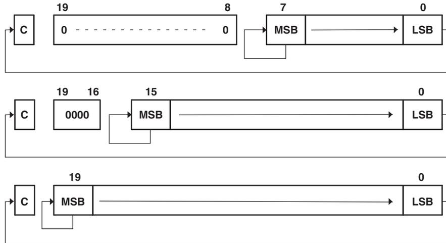
Figure 4-47. Rotate Right Arithmetically RRAX(.B,.A) – Register Mode
