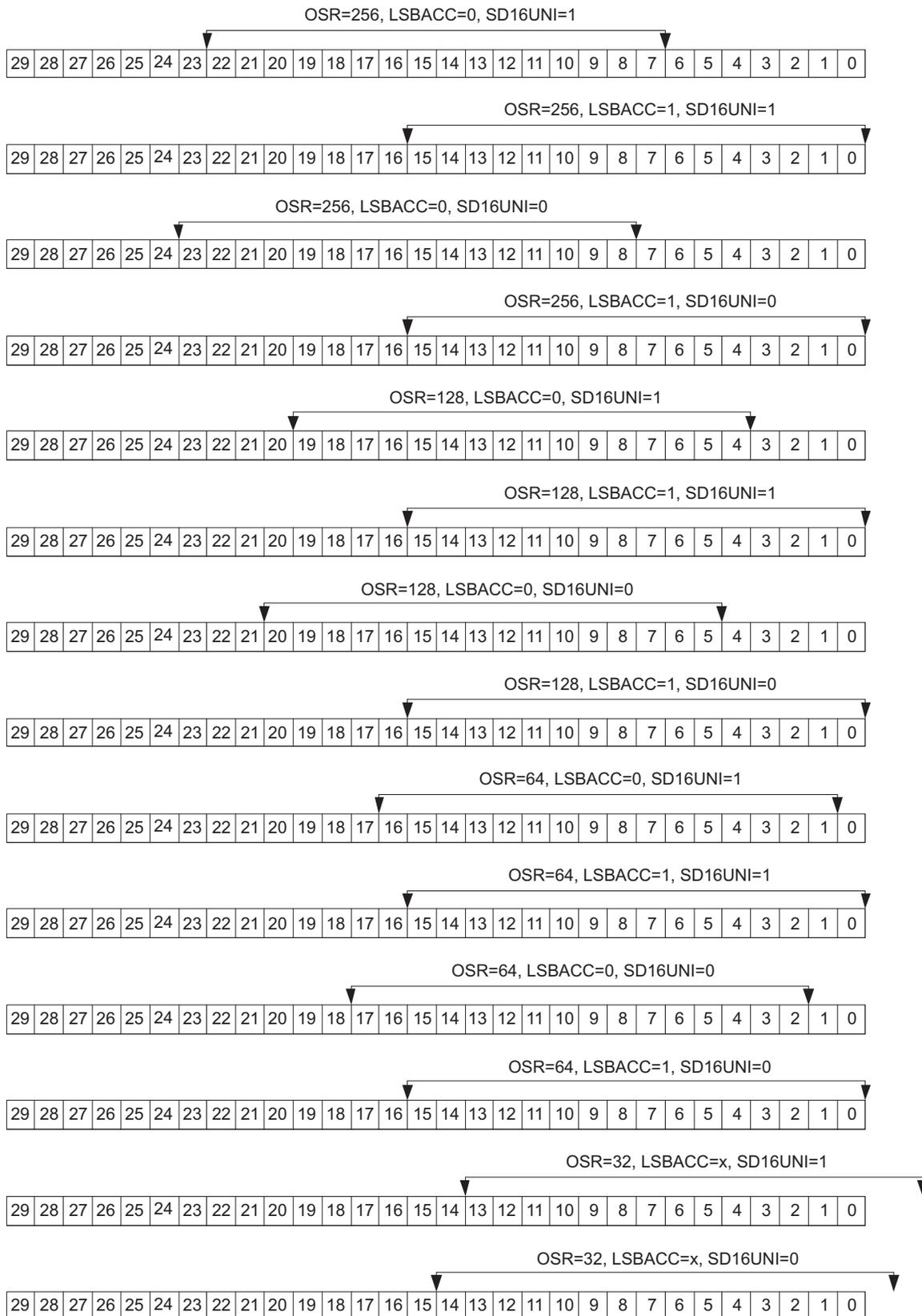
Figure 26-5. Used Bits of Digital Filter Output
