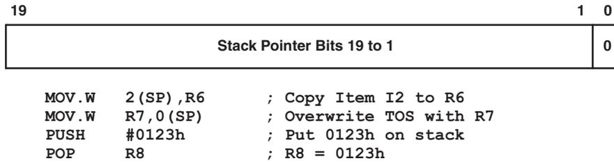
Figure 4-5. Stack Pointer
