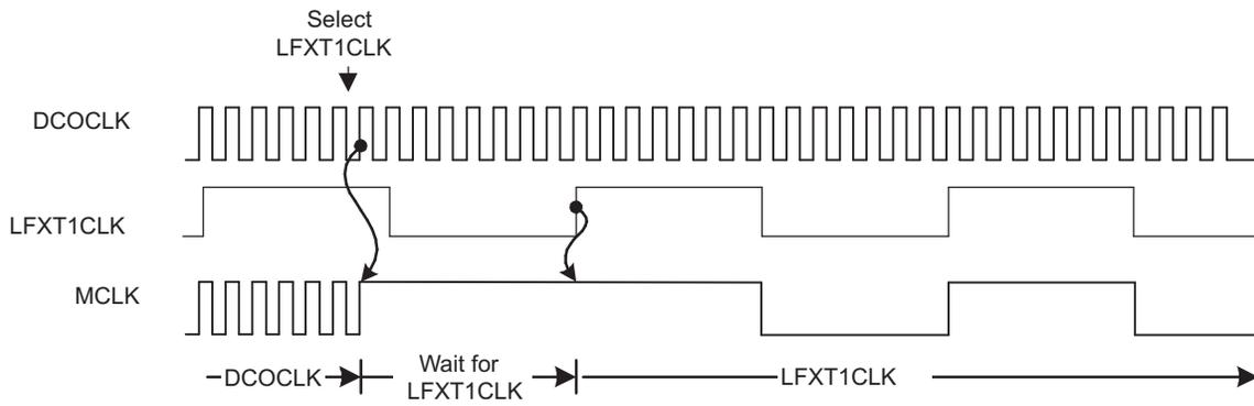
**Figure 5-9. Switch MCLK from DCOCLK to LFXT1CLK**
