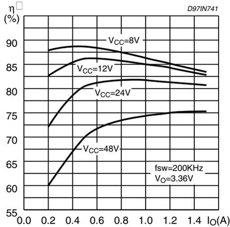
Figure 20. Efficiency vs. V<sub>CC</sub>.
