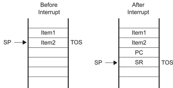
**Figure 2-6. Interrupt Processing**
