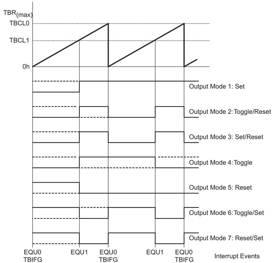
Figure 13-12. Output Example, Timer in Up Mode
