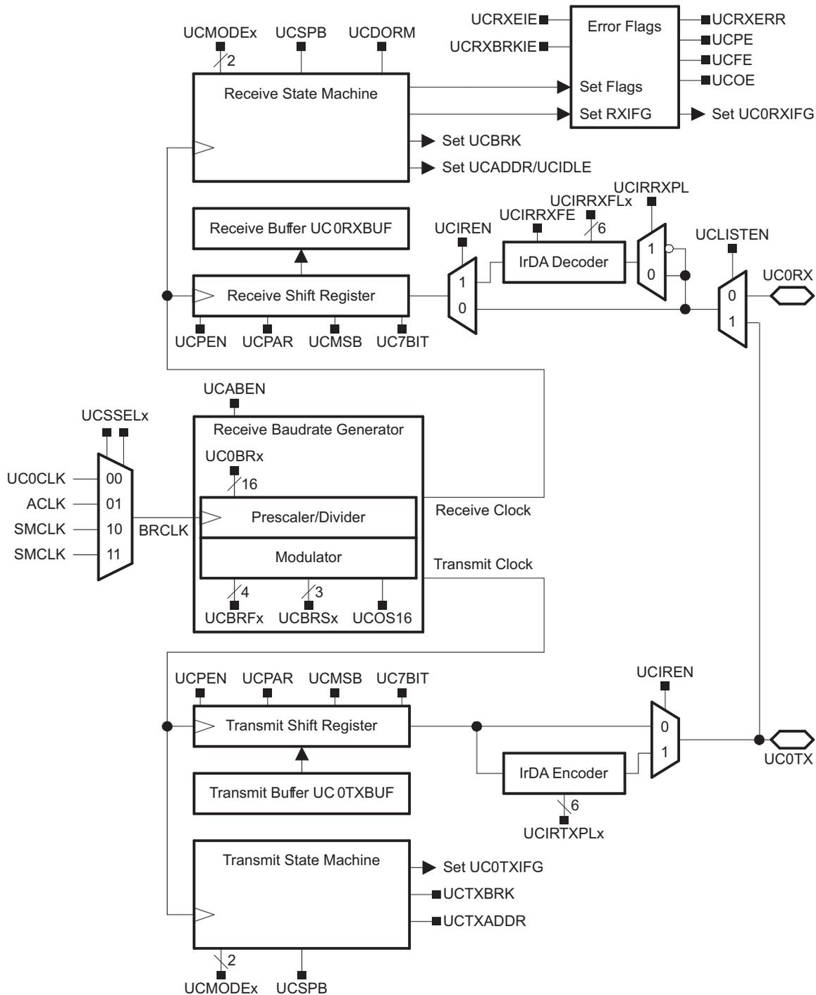
Figure 15-1. USCI\_Ax Block Diagram: UART Mode (UCSYNC = 0)
