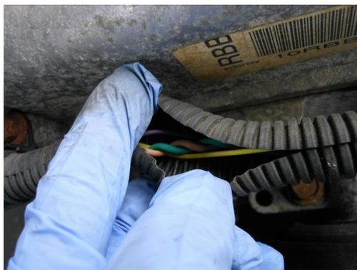
*Further up the wire sleeve, where the wires are not chewed. Here I can cut them and solder new wires in.*
