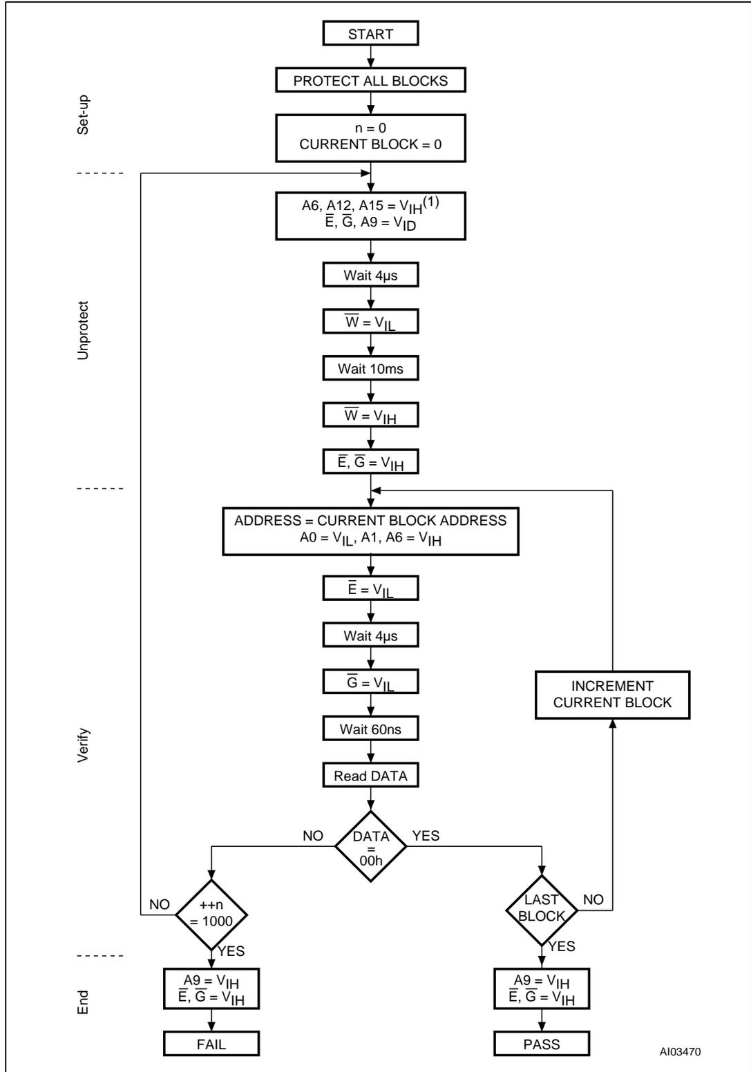
Figure 20. In-system equipment block protect flowchart
