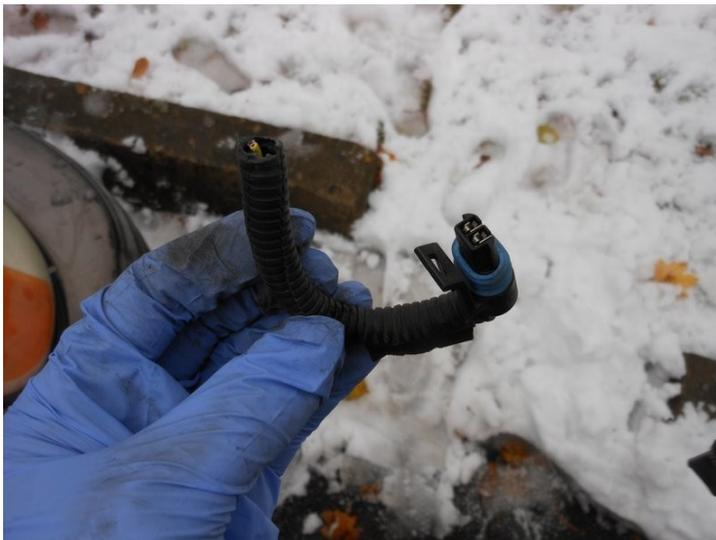
*End of the connector from wire that was chewed. Lucky for me, the connector was intact.*
