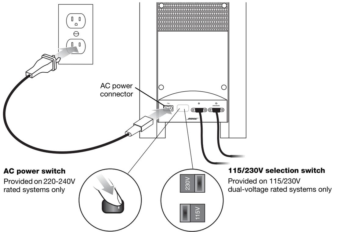
**Note:** Bose recommends using a safety agency-approved surge protector on all electronic equipment. Voltage variations and spikes can damage electronic components in any system. A quality suppressor can eliminate the vast majority of failures attributed to surges and may be purchased at electronics stores.
