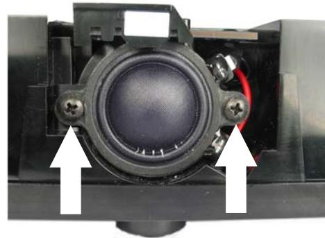
Figure 8. Front Tweeter Removal
