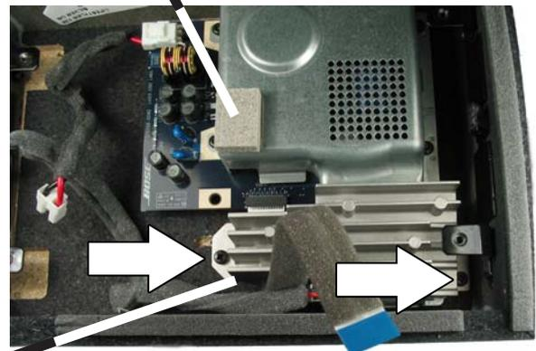
Figure 21. Heat Sink Removal
