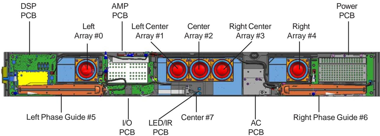
Figure 26. Transducer and PCB Identification
