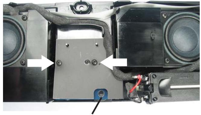
Align AC PCB insulator with top cover screw hole
