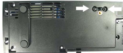
Figure 4. Phase Guide Speaker Screws
