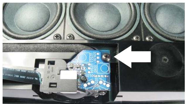
Figure 14. IR/LED PCB
