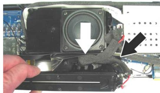
Figure 5. Phase Guide Wire Routing
