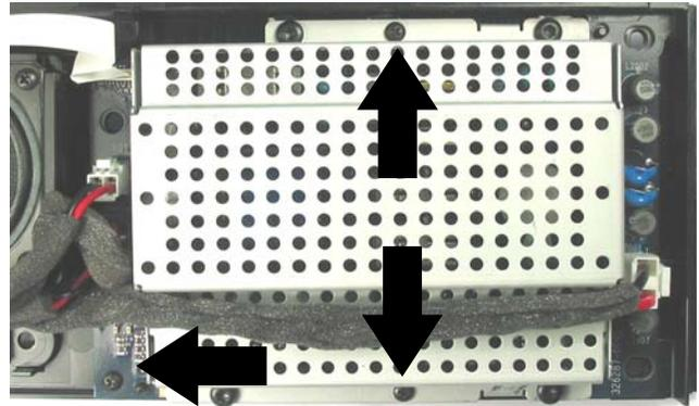
**Figure 16. Power Supply PCB Removal**
