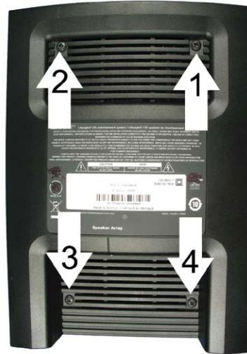
Figure 17. Rear Cover Removal
