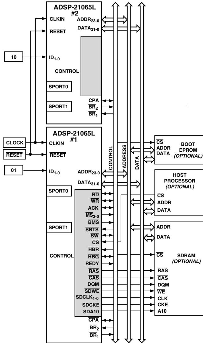
Figure 3. Multiprocessing System
