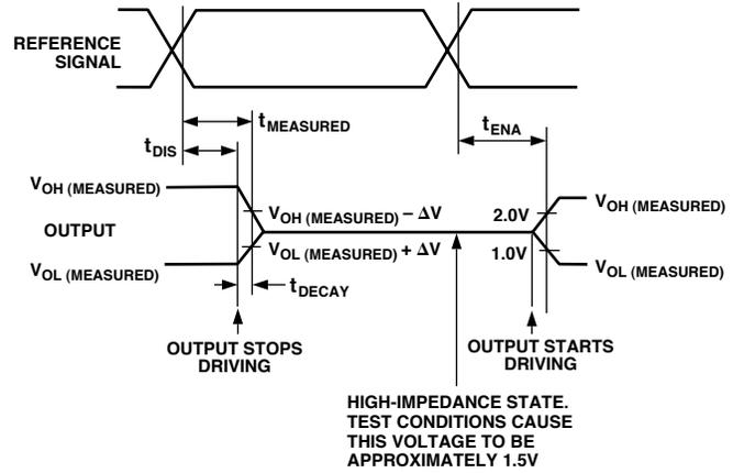
Figure 25. Output Enable
