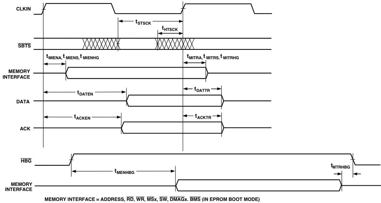
Figure 17. Three-State Timing
