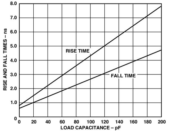
Figure 29. Typical Rise and Fall Time (0.8 V–2.0 V)
