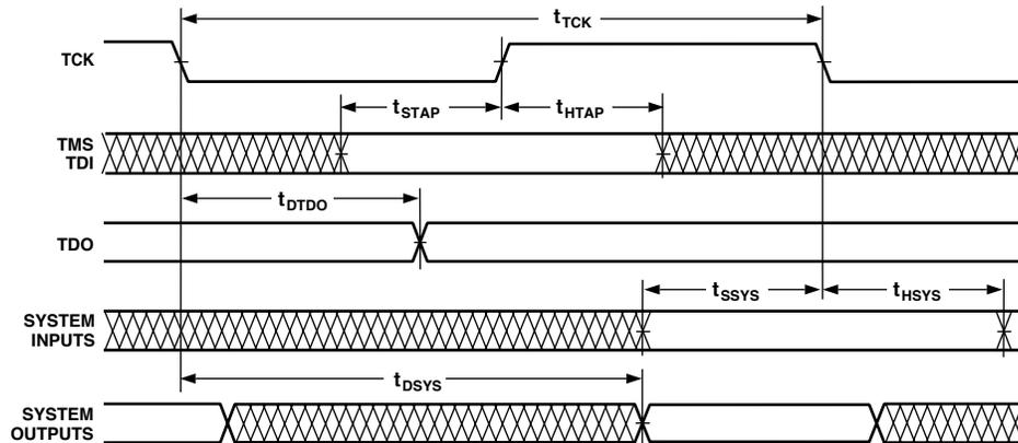
Figure 23. JTAG Test Access Port and Emulation
