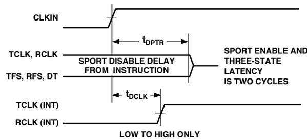
Figure 20. Serial Ports
