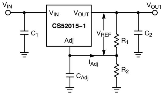
Figure 11. Resistor Divider Scheme
