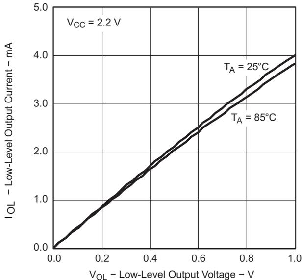
Figure 16. USI Low-Level Output Voltage vs Output Current
