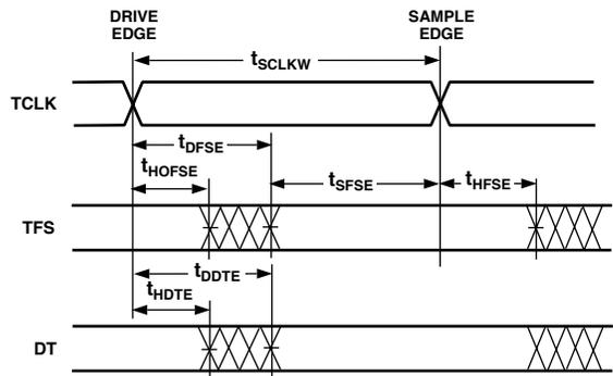
NOTE: EITHER THE RISING EDGE OR FALLING EDGE OF RCLK OR TCLK CAN BE USED AS THE ACTIVE SAMPLING EDGE.
