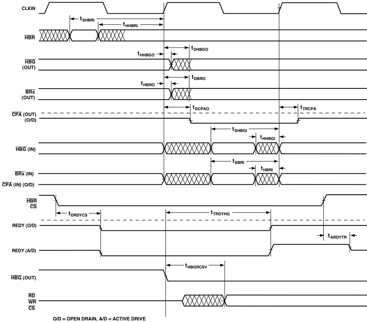
Figure 15. Multiprocessor Bus Request and Host Bus Request
