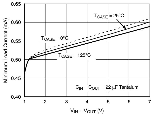
Figure 6. Minimum Load Current vs.  $V_{IN} - V_{OUT}$
