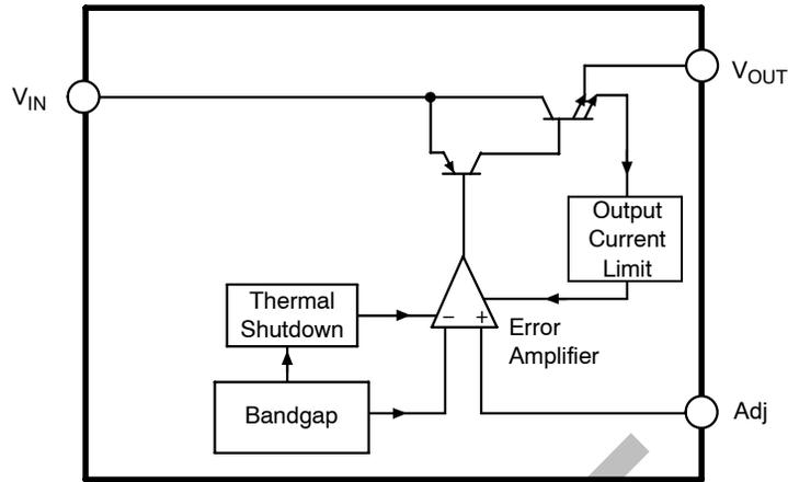
Figure 2. Block Diagram
