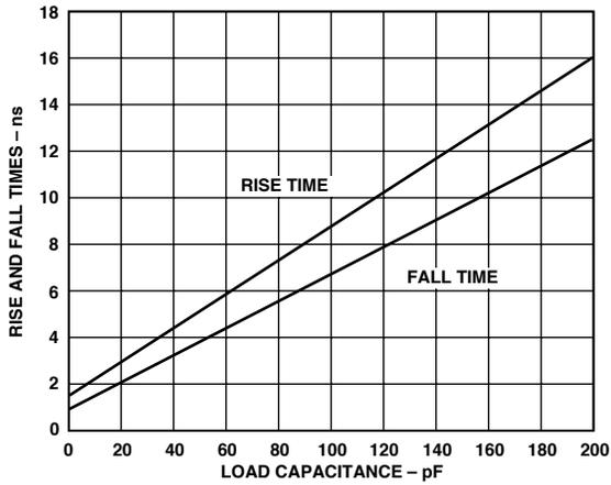
Figure 28. Typical Rise and Fall Time (10%–90% V<sub>DD</sub>)
