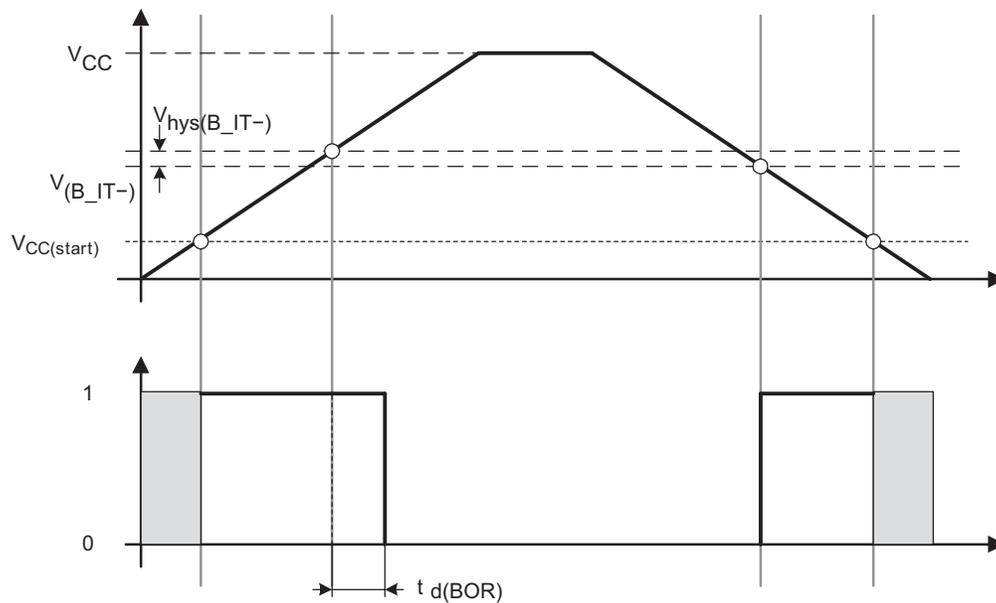
Figure 12. POR/Brownout Reset (BOR) vs Supply Voltage
