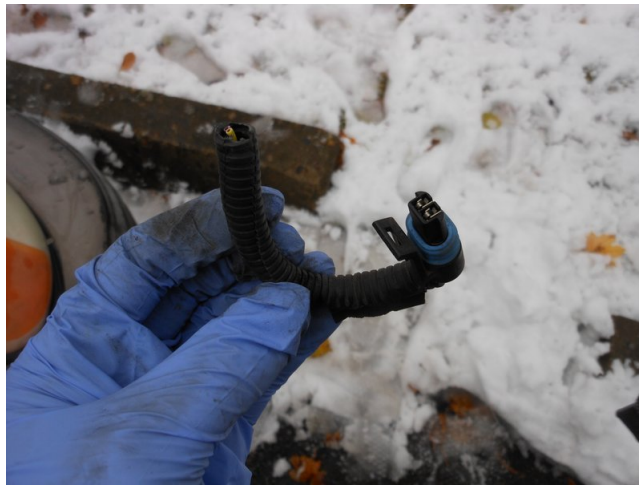
Figure 1: Cut off the connector at one end, so I can attach wires to it. This is what connected to the transmission
