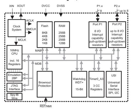
Note: Port P2. Two pins are available on the 14/16-pin package options. Eight pins are available on the 20-pin package options.
