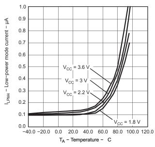
Figure 5. LPM4 Current vs Temperature
