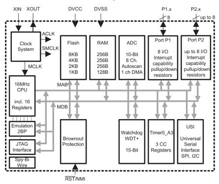
Note: Port P2. Two pins are available on the 14/16-pin package options. Eight pins are available on the 20-pin package options.
