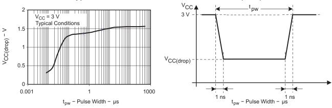
Figure 13.  $V_{CC(drop)}$  Level With a Square Voltage Drop to Generate a POR/Brownout Signal
