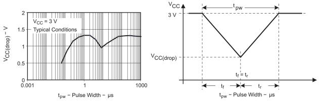
Figure 14. V<sub>CC(drop)</sub> Level With a Triangle Voltage Drop to Generate a POR/Brownout Signal
