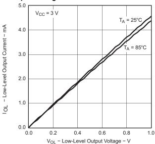
Figure 17. USI Low-Level Output Voltage vs Output Current
