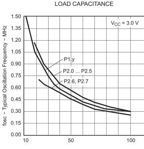
C<sub>LOAD</sub> - External Capacitance - pF Figure 11.
