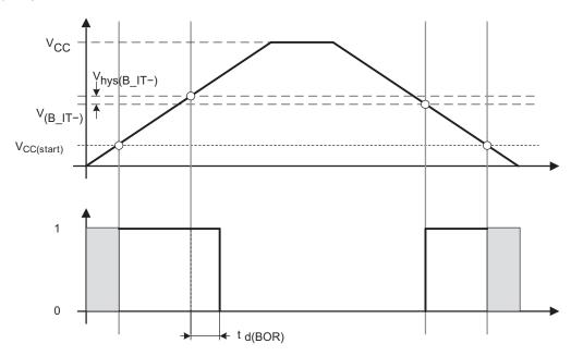
Figure 12. POR/Brownout Reset (BOR) vs Supply Voltage
