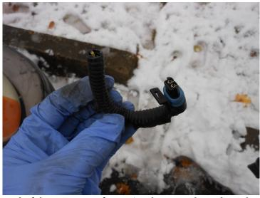
End of the connector from wire that was chewed. Lucky for me, the connector was intact.
