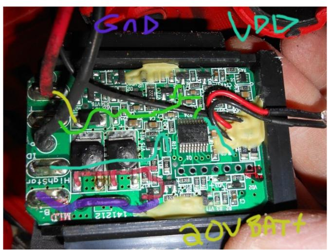
Board. When switch is pressed, there is 20V on the tab of vreg. I believe the VReg must've overheated and shorted (perhaps counterfeit?). Original device must've been an adjustable vreg, per the resistors on the red line for adj. pin. Pin out is Tab = VIN, Left pin = Adj, ? Though Right pin is to GND. Maybe it's a current limiter, not an adjustable Vreg, allowing Tab when V+ to be dropped down and current will flow. In that respect, maybe these are power transistors. Not Vregs.
