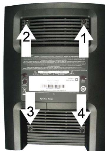
**Figure 17. Rear Cover Removal**
