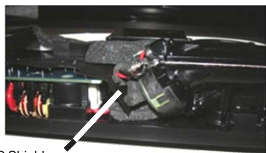
Figure 6. Right Phase Guide Wire Routing
