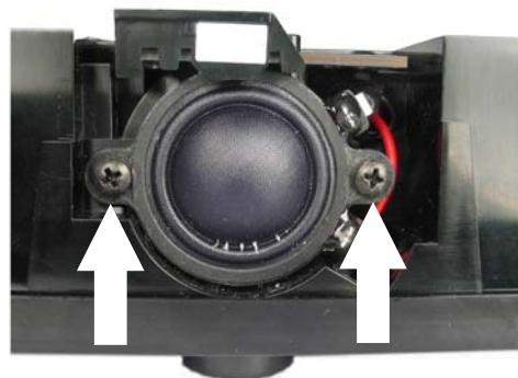
Figure 8. Front Tweeter Removal
