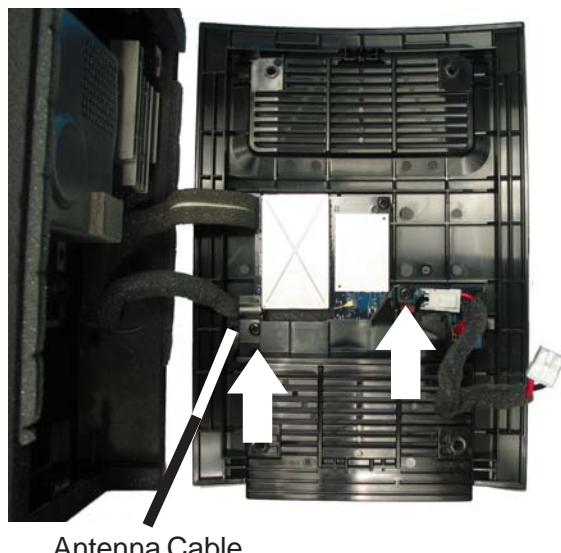
**Figure 19. Connector Cover Removal**
