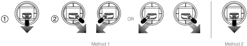
**⚠ DO NOT perform the CSC command when the aircraft is flying in mid-air.**
