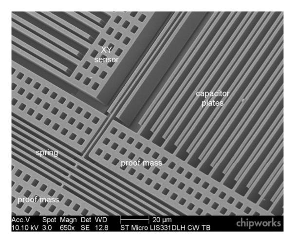
This is just one small part of a MEMS device – the fingers that you see are pushed in one direction or the other by g-forces (movement of your drone, the wind, etc.) and send electrical signals detailing the exact forces and direction of them back to a computer inside the gimbal controller.
