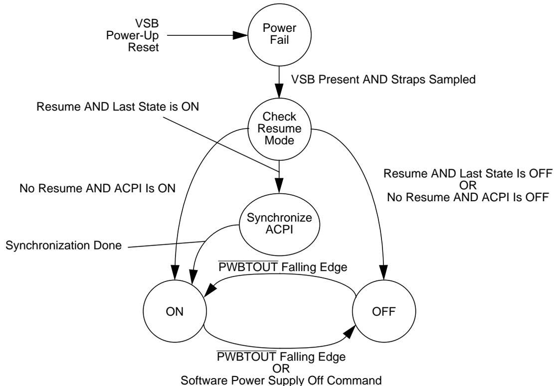
**Figure 4. Legacy Power Supply Control State Diagram**
