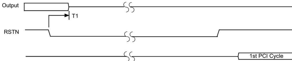
Note: Minimum reset-complete time is a function of the PCI-, transmit-, and receive-clock frequencies.
