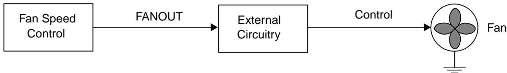
Figure 13. Fan Speed Control - System Configuration
