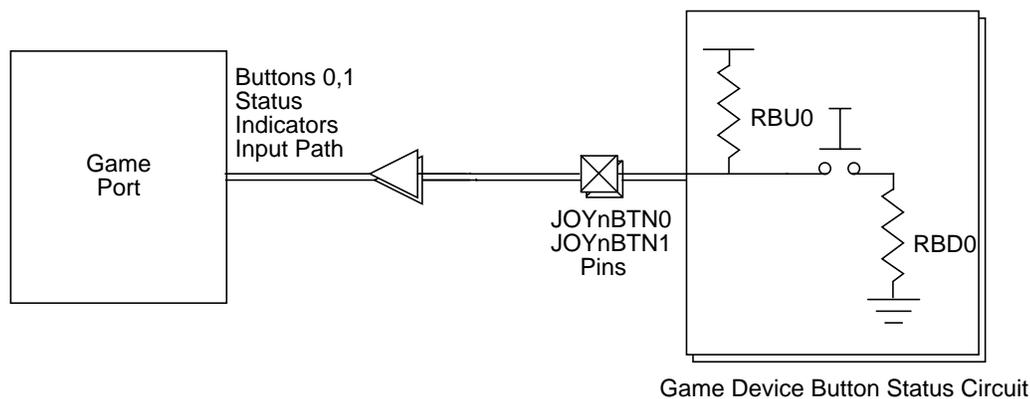
Figure 30. Game Device Button Status Indication Mechanism
