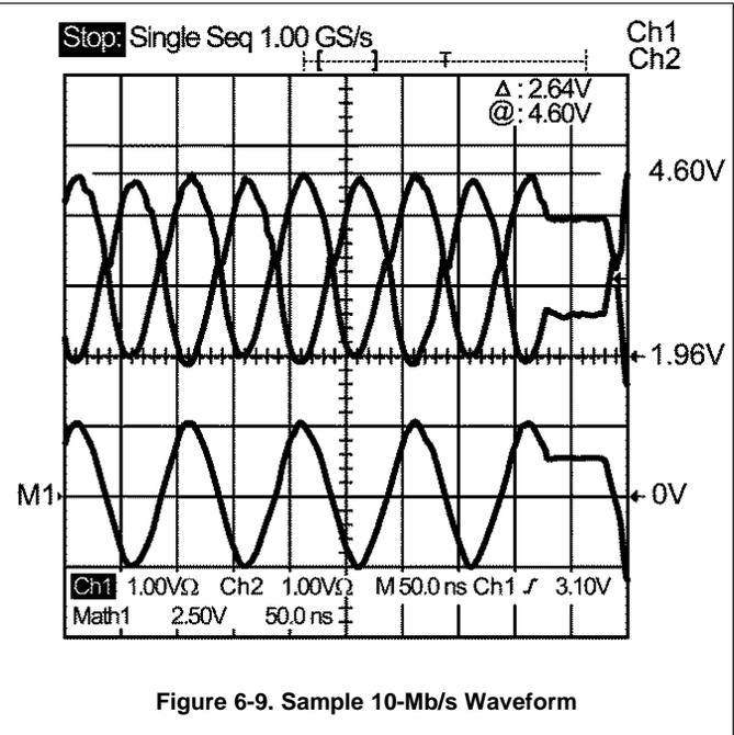
Figure 6-9. Sample 10-Mb/s Waveform
