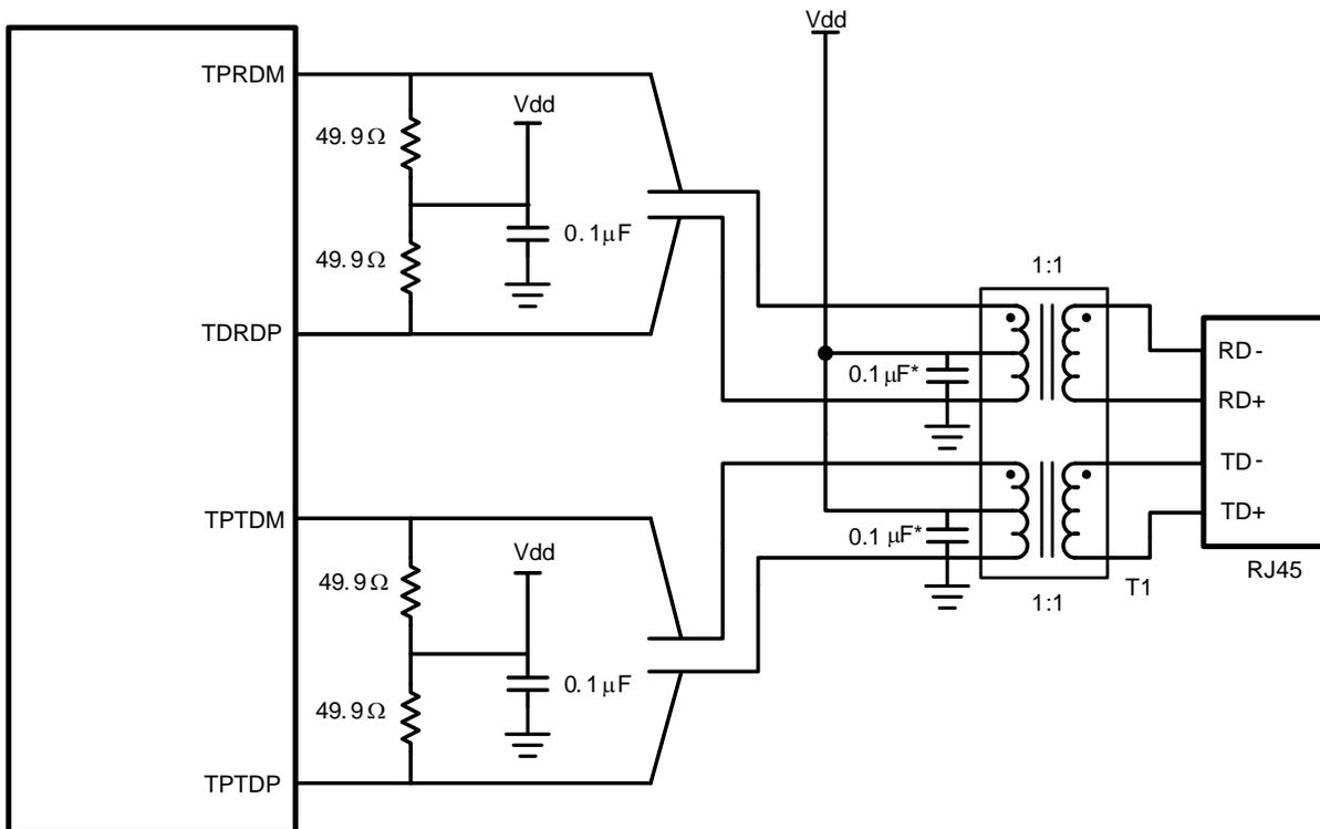
\* Place capacitors close to the transformer center taps.
