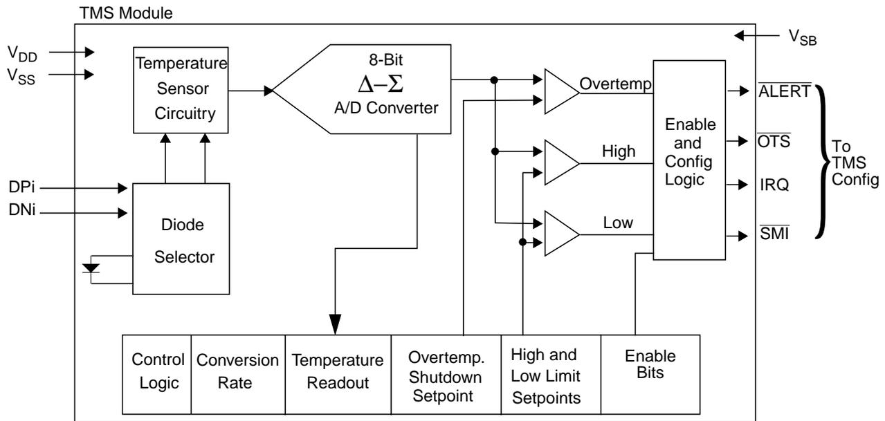
Figure 41. TMS Simplified Block Diagram
