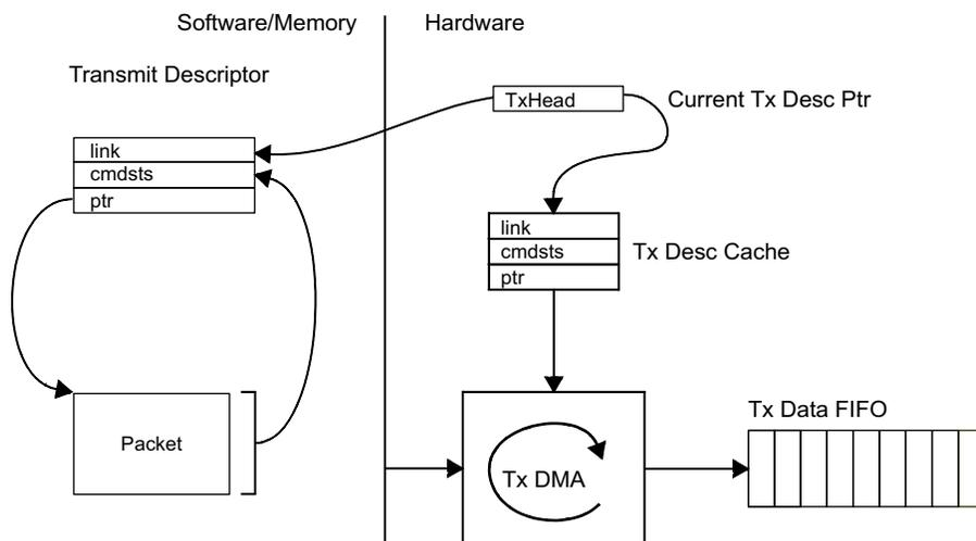
Figure 5-20. Transmit Architecture
