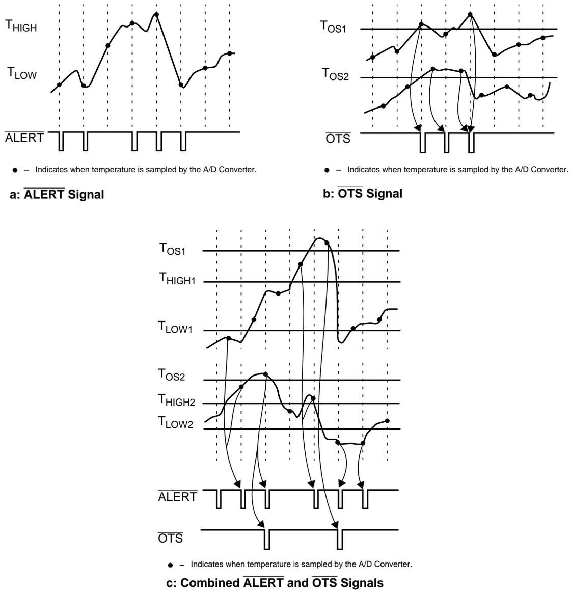
**Figure 43. OTS and ALERT Temperature Response Diagrams**
