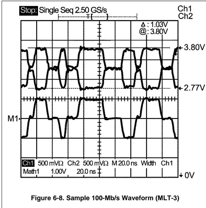
Figure 6-8. Sample 100-Mb/s Waveform (MLT-3)
