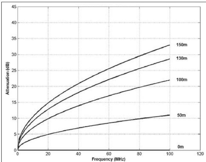
Figure 5-10. EIA/TIA Attenuation vs Frequency for 0, 50, 100, 130 and 150 Meters of CAT V Cable
