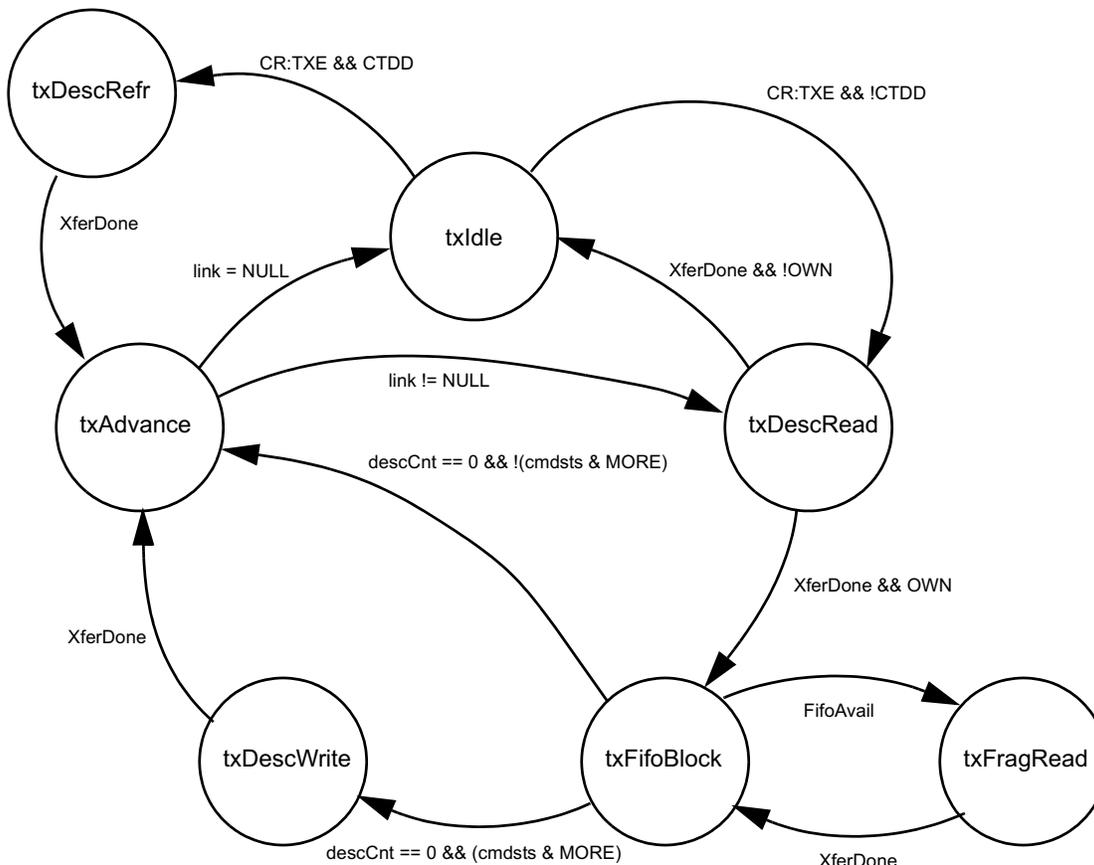
Figure 5-21. Transmit State Diagram
