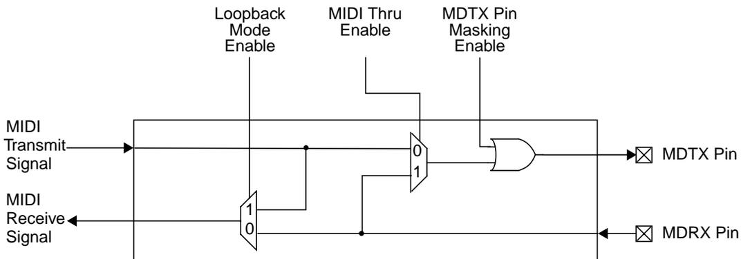
Figure 34. MIDI Signals Routing Control Logic
