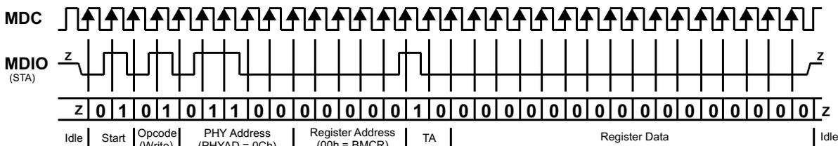
Figure 5-5. Typical MDC and MDIO Write Operation
