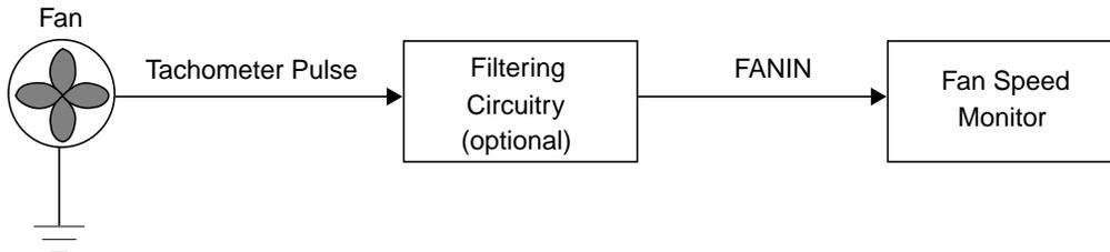
Figure 15. Fan Speed Monitor - System Configuration
