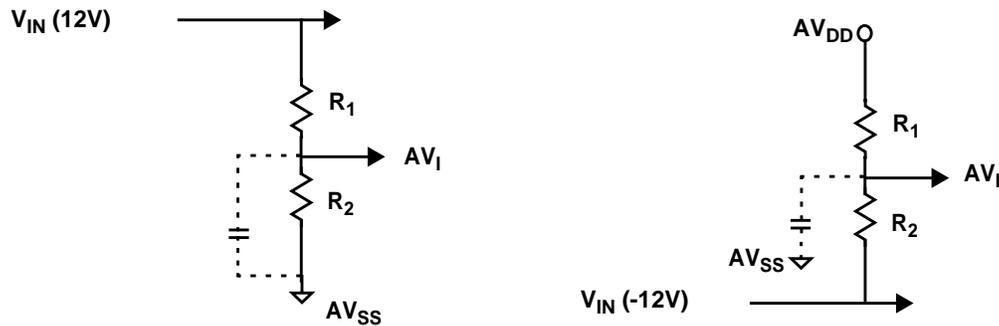
Figure 40. Measurement Out of Positive and Negative Voltages
