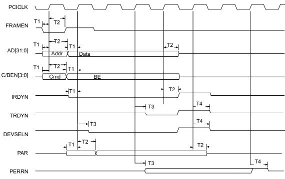
Figure 4-11. PCI Target Write (see PCI BUS CYCLES in Section 4.6)
