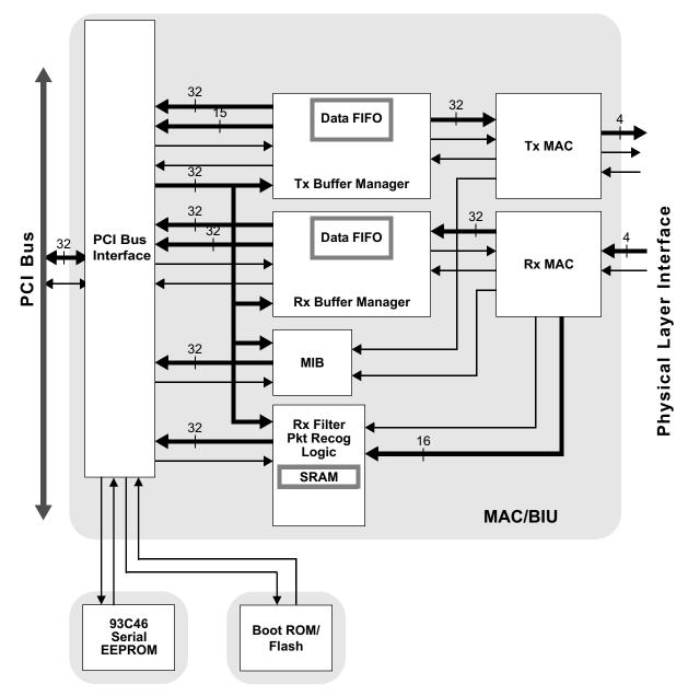
Figure 5-2. MAC and BIU Functional Block Diagram
