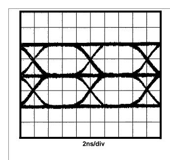
Figure 5-12. MLT-3 Signal Measured at All After 50 Meters of CAT V Cable
