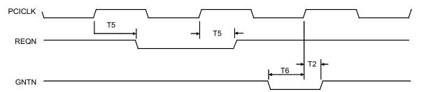
Figure 4-14. PCI Bus Arbitration (see PCI BUS CYCLES in Section 4.6)
