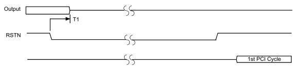
Note: Minimum reset-complete time is a function of the PCI-, transmit-, and receive-clock frequencies.
