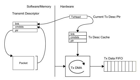
Figure 5-20. Transmit Architecture
