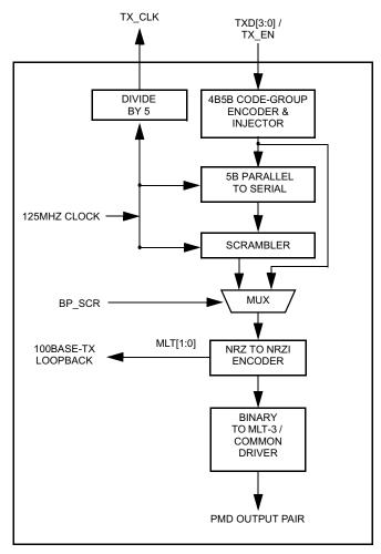
Figure 5-6. 100BASE-TX Transmit Block Diagram
