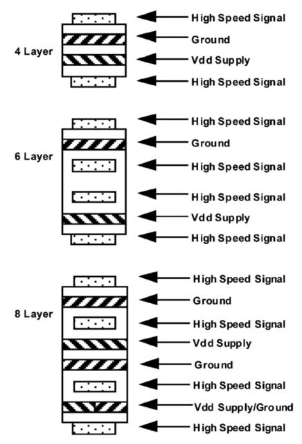
Figure 8-3. PCB Stripline Layer Stacking
