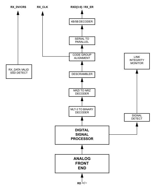
Figure 5-8. 100BASE-TX Receive Block Diagram
