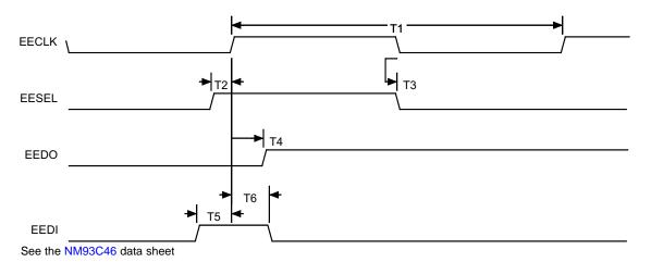
Figure 4-15. EEPROM Auto-Load (see EEPROM AUTO-LOAD in Section 4.6)
