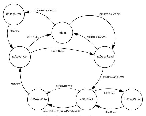
Figure 5-23. Receive State Diagram
