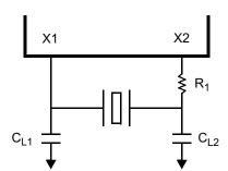
Figure 6-3. Crystal Oscillator Circuit
