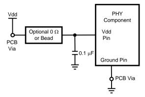
Figure 7-1. V<sub>DD</sub> Bypass Layout
