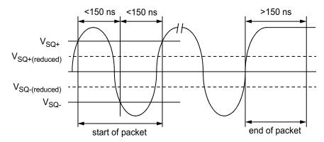
Figure 5-14. 10BASE-T Twisted Pair Smart Squelch Operation
