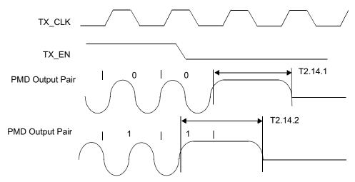
Figure 4-18. 10BASE-T Transmit End of Packet (see 10BASE-T TRANSMIT END OF PACKET in Section 4.6)
