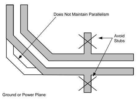
Figure 8-2. Differential Signal Pair-Plane Crossing
