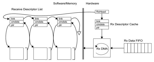
Figure 5-22. Receive Architecture
