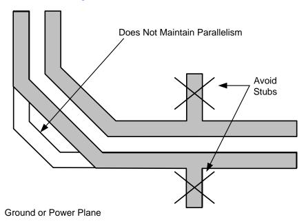
Figure 8-1. Differential Signal Pair - Stubs
