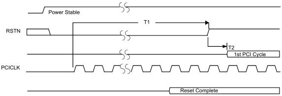
Note: Minimum reset complete time is a function of the PCI-, transmit-, and receive-clock frequencies.
