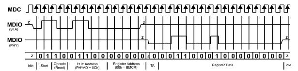
Figure 5-4. Typical MDC and MDIO Read Operation
