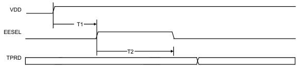
Figure 4-5. POR PCI Inactive (see POR PCI INACTIVE in Section 4.6)
