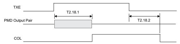
Figure 4-19. 10-Mb/s Jabber Timing (see 10-Mb/s JABBER TIMING in Section 4.6)
