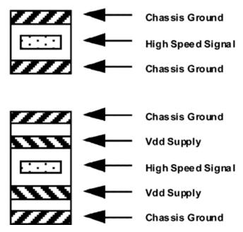
Figure 8-4. Alternative PCB Stripline Layer Stacking
