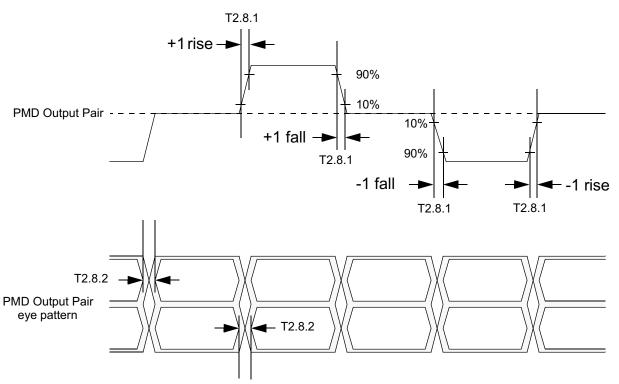
Note: Normal mismatch is the difference between the maximum and minimum of all rise and fall times.
