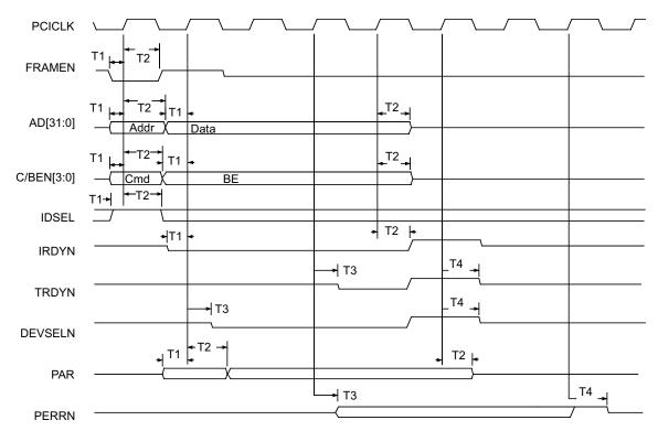
Figure 4-7. PCI Configuration Write (see PCI BUS CYCLES in Section 4.6)
