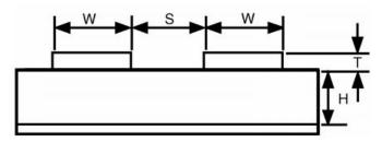
$W = \mbox{Width of the trace} \\ H = \mbox{Height of dielectric above the return plane}$
