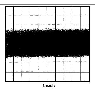
Figure 5-13. MLT-3 Signal Measured at All After 100 Meters of CAT V Cable
