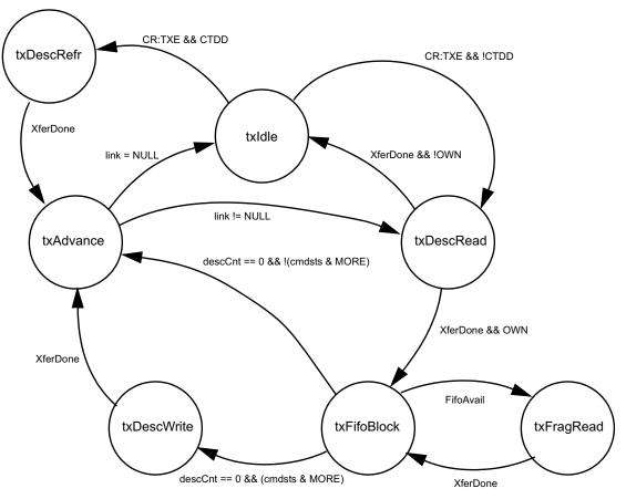
Figure 5-21. Transmit State Diagram
