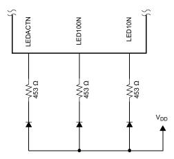
Figure 5-3. LED Loading Example
