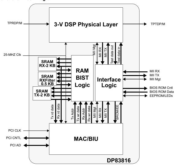
Figure 5-1. DP83816 Functional Block Diagram
