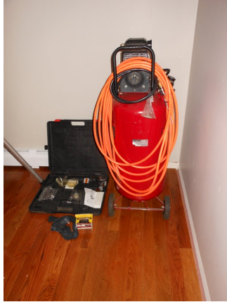
Figure 14: Air compressor (oversized for this task)
