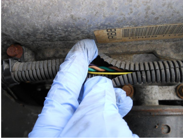
Figure 3: Further up the wire sleeve, where the wires are not chewed. Here I can cut them and solder new wires in. There are four wires here, as the sleeve was used for multiple wires.
