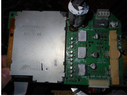
Figure 1: Main Board. CPU / ADC is under shield.
