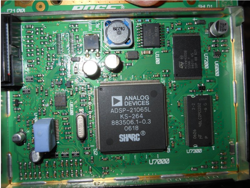
Figure 2: Main CPU board under can. Starting from 12 o'clock going clockwise, Linear and Switching power regulator, Flash, RAM, ADSP CPU (SHARC), ADC (under blue foam).
