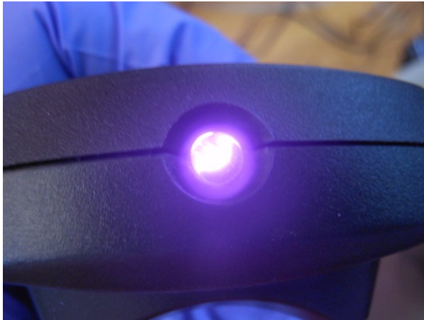
Figure 5: IR is normally invisible, however my digital camera picks it up. A Quick way to test IR is to take a picture. Alternatively, you can probe the diode leads with an oscilloscope.
