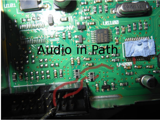
Figure 3: Audio In Path to the ADC
