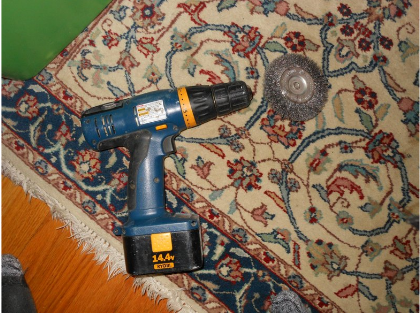
Figure 3: This wire wheel easily scraps off mortar or concrete Shows a small wire wheel you can use on the end of a drill. This can be used to sand away areas of concrete or mortar that aren't flat. I should've used this more before I put down the original layer of thinset mortar, before the membrane was down, but because I didn't, I had a non level plane at the end. As this was a closet no big deal, but it didn't look 100 Surface must be flat!!!! Very important.
