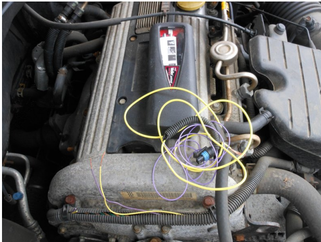
Figure 4: With portable soldering iron (portasol butane powered) and some wire, this is an easy fix. A little scary, though, being close to the gas line. Even if gas burns not explodes I don't want any surprises. I made sure nothing was open, exposed, or leaking. Be careful out there!
