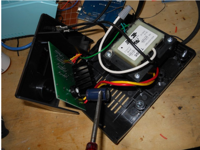
Figure 1: The board is a large power transistor with a Pic to control it. Here I added a capacitor per some online guides, but no dice. It turned out to be a failed iron.
