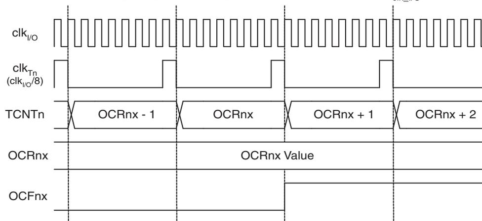
Figure 20-11 shows the setting of OCF2A and the clearing of TCNT2 in CTC mode.
