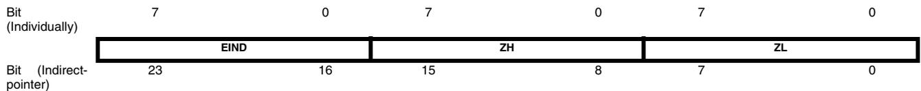
The actual number of bits is implementation dependent. Unused bits in an implementation will always read as zero. For compatibility with future devices, be sure to write these bits to zero.
