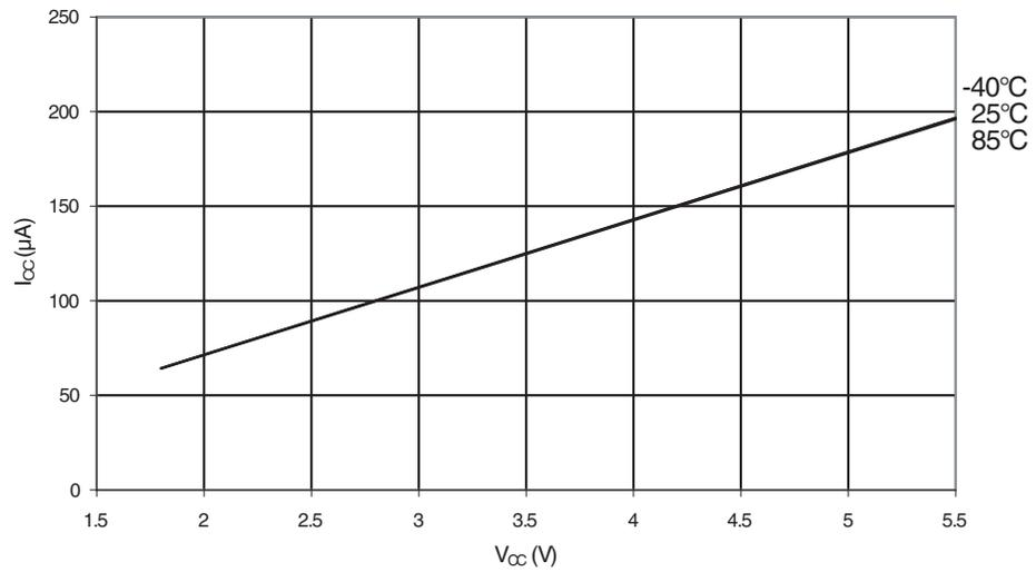
**Figure 32-43.** Watchdog Timer Current vs.  $V_{CC}$
