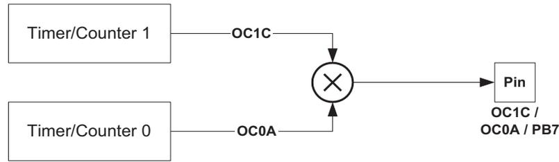
When the modulator is enabled, the two output compare channels are modulated together as shown in the block diagram (see Figure 19-1).
