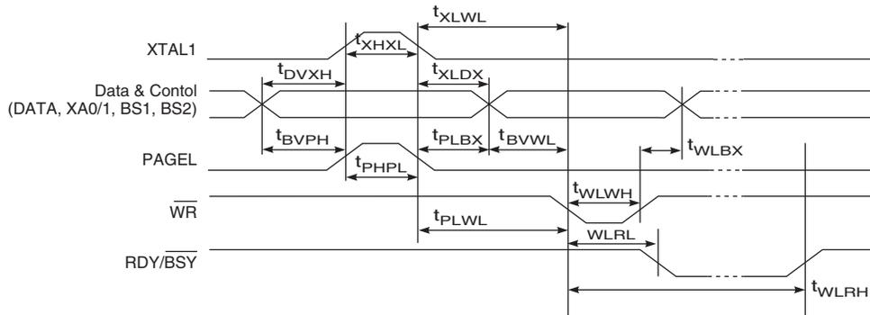
**Figure 30-8.** Parallel Programming Timing, Loading Sequence with Timing Requirements<sup>(1)</sup>
