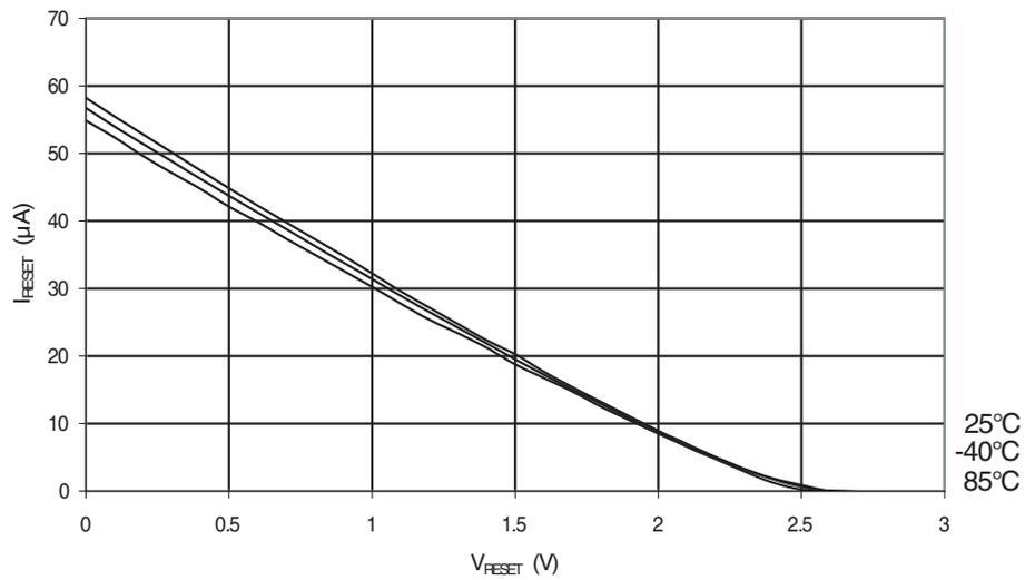
**Figure 32-21.** Reset Pull-up Resistor Current vs. Reset Pin Voltage ( $V_{CC} = 5V$ )
