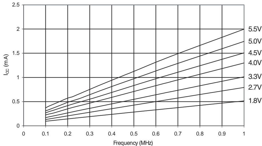
**Figure 32-2.** Active Supply Current vs. Frequency (1MHz - 16MHz)
