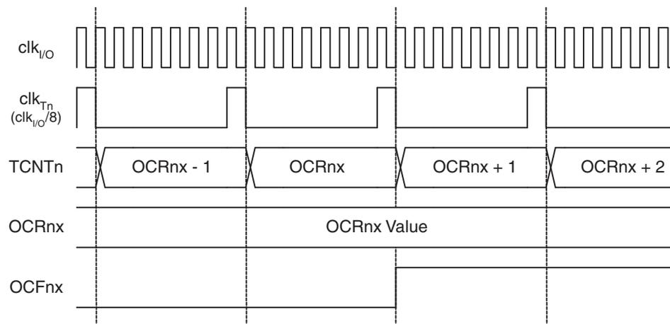
Figure 17-12 shows the count sequence close to TOP in various modes. When using phase and frequency correct PWM mode the OCRnx Register is updated at BOTTOM. The timing diagrams will be the same, but TOP should be replaced by BOTTOM, TOP-1 by BOTTOM+1 and so on. The same renaming applies for modes that set the TOVn Flag at BOTTOM.
