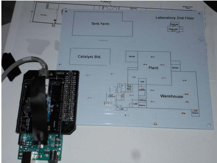
Figure 5: Revision 2 build, with Map PCB
