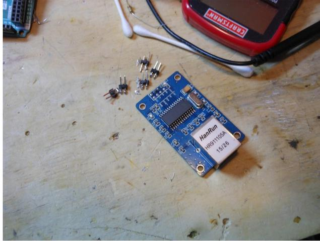
Figure 3: Cut plastic part off in pairs, then desolder. OR, design your board so you don't have to remove the pin headers!
