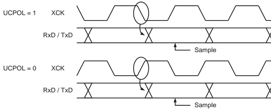
The UCPOLn bit UCRSC selects which XCKn clock edge is used for data sampling and which is used for data change. As [Figure 22-3](#) shows, when UCPOLn is zero the data will be changed at rising XCKn edge and sampled at falling XCKn edge. If UCPOLn is set, the data will be changed at falling XCKn edge and sampled at rising XCKn edge.
