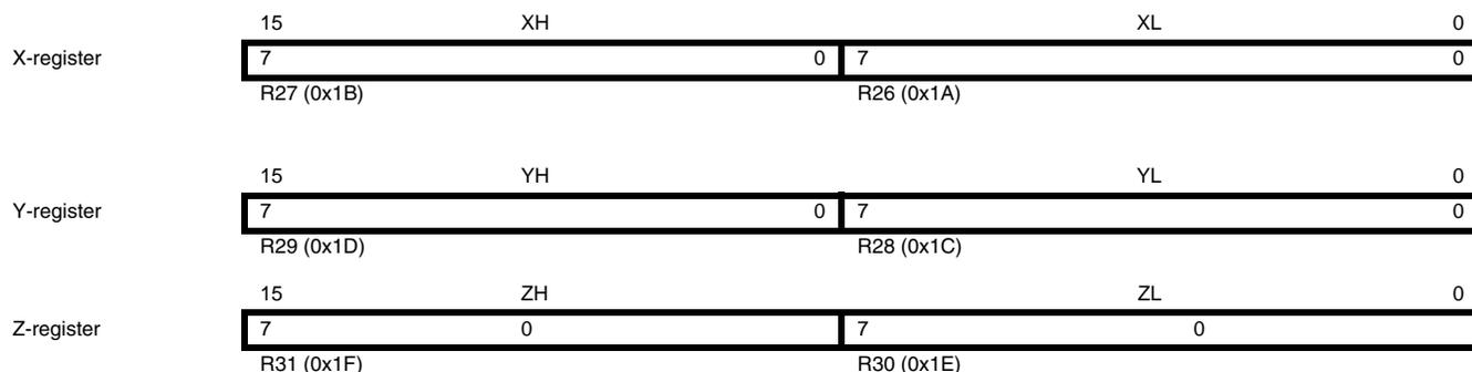
In the different addressing modes these address registers have functions as fixed displacement, automatic increment, and automatic decrement (see the “Instruction Set Summary” on page 404 for details).
