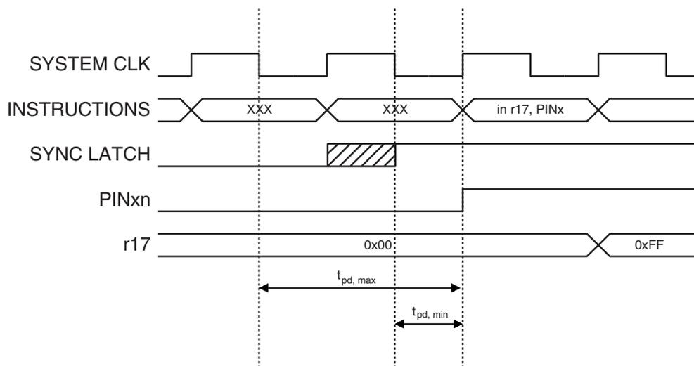
Consider the clock period starting shortly after the first falling edge of the system clock. The latch is closed when the clock is low, and goes transparent when the clock is high, as indicated by the shaded region of the "SYNC
