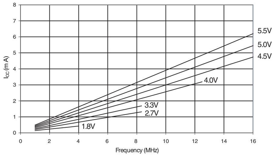
**Figure 32-8.** Idle Supply Current vs.  $V_{CC}$  (Internal RC Oscillator, 8MHz)
