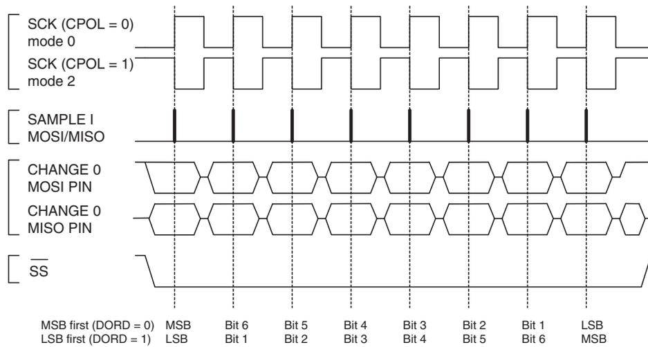
**Figure 21-4. SPI Transfer Format with CPHA = 1**
