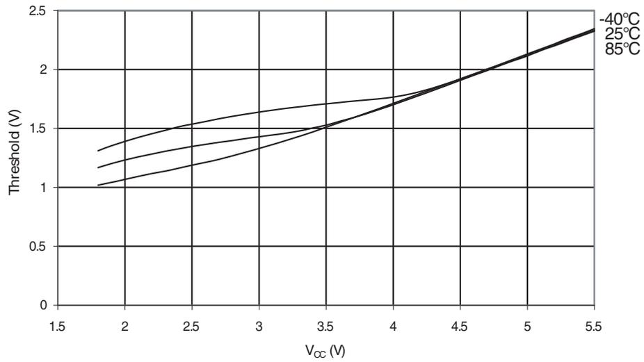
**Figure 32-30.** Reset Input Threshold Voltage vs.  $V_{CC}$  ( $V_{IL}$ , IO Pin Read as “0”)
