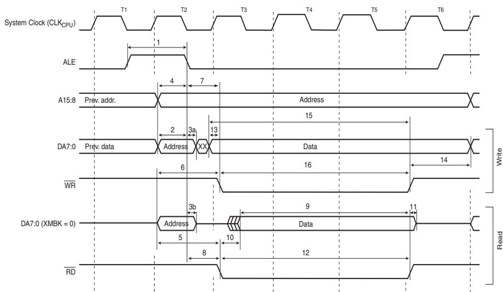
**Figure 31-12. External Memory Timing (SRWn1 = 1, SRWn0 = 1)<sup>0</sup>**
