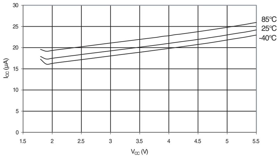
**Figure 32-41.** ADC Current vs.  $V_{CC}$  (AREF =  $AV_{CC}$ )
