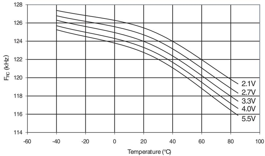
**Figure 32-37.** Calibrated 8MHz RC Oscillator Frequency vs.  $V_{CC}$
