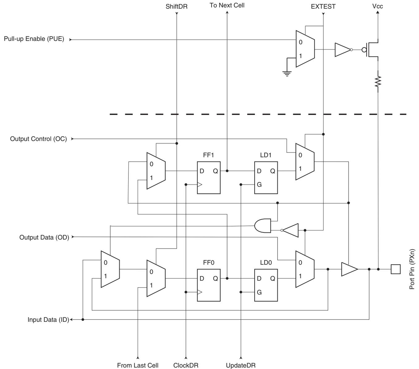
**Figure 28-4.** General Port Pin Schematic Diagram
