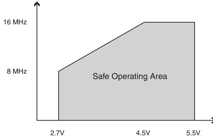
**Figure 31-4.** Maximum Frequency vs.  $V_{CC}$ , ATmega2560/ATmega2561
