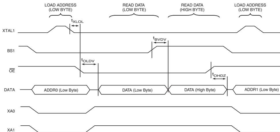
Note: 1. The timing requirements shown in Figure 30-7 (that is,  $t_{DVXH}$ ,  $t_{XHL}$ , and  $t_{XLDX}$ ) also apply to reading operation.
