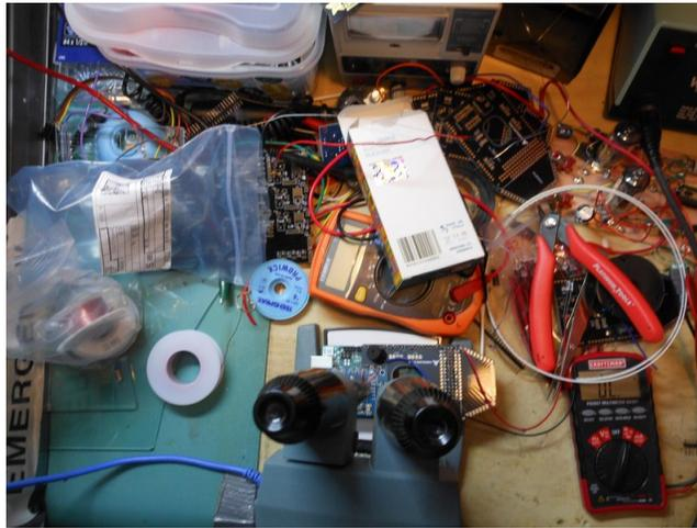
Figure 4: If you are going to be soldering high gauge magnet wire, you should use a microscope. It makes the process much more enjoyable, and efficient.
