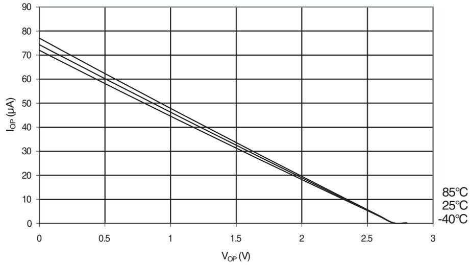
**Figure 32-18.** I/O Pin Pull-up Resistor Current vs. Input Voltage ( $V_{CC} = 5V$ )
