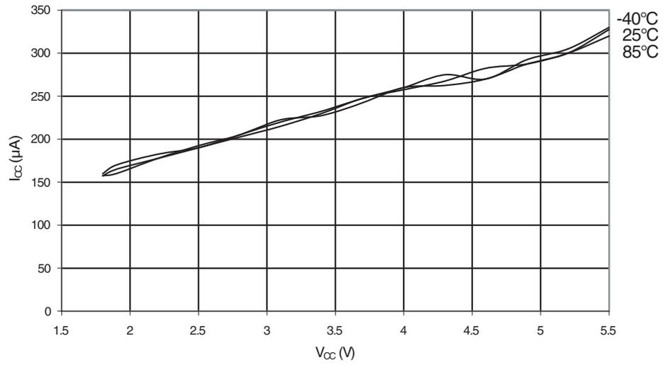
**Figure 32-42.** AREF External Reference Current vs.  $V_{CC}$
