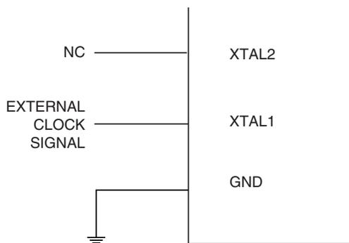
When this clock source is selected, start-up times are determined by the SUT Fuses as shown in [Table 10-15](#) on [page 49](#).
