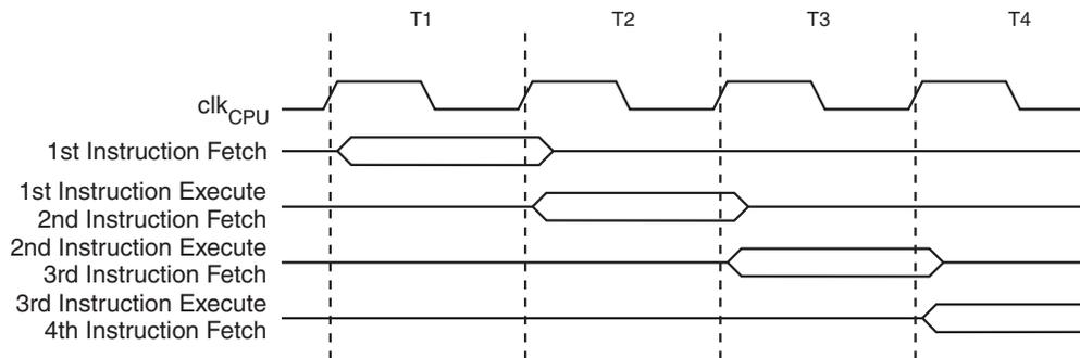
Figure 7-7 shows the internal timing concept for the Register File. In a single clock cycle an ALU operation using two register operands is executed, and the result is stored back to the destination register.
