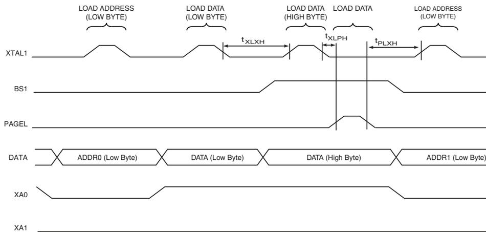
Note: 1. The timing requirements shown in Figure 30-7 (that is,  $t_{DVXH}$ ,  $t_{XHL}$ , and  $t_{XLDX}$ ) also apply to loading operation.
