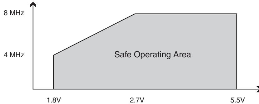
Figure 31-2. Maximum Frequency vs.  $V_{CC}$  when also No-Read-While-Write Section<sup>(1)</sup>, ATmega2560V/ATmega2561V, is used
