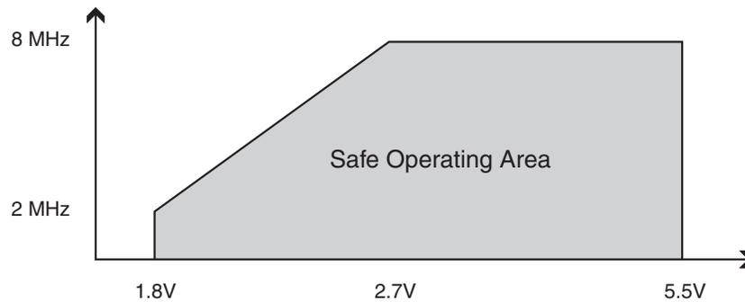
Note: 1. When only using the Read-While-Write Section of the program memory, a higher speed can be achieved at low voltage, see “Read-While-Write and No Read-While-Write Flash Sections” on page 310 for addresses.
