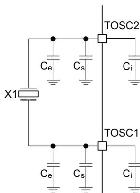
To find suitable load capacitance for a 32.768kHz crystal, consult the crystal datasheet.
