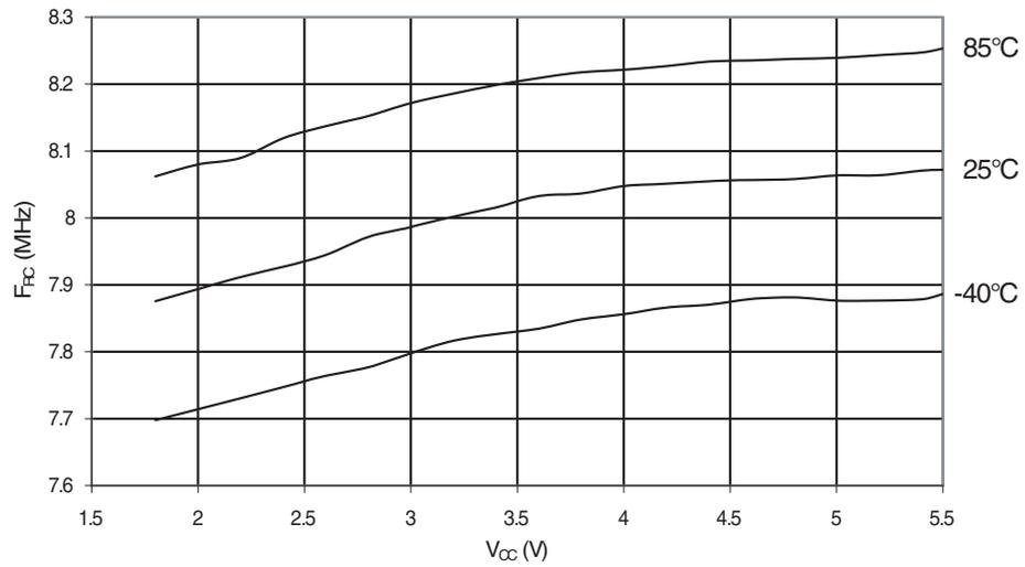
**Figure 32-38.** Calibrated 8MHz RC Oscillator Frequency vs. Temperature
