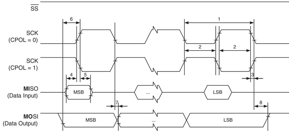
**Figure 31-8. SPI Interface Timing Requirements (Slave Mode)**
