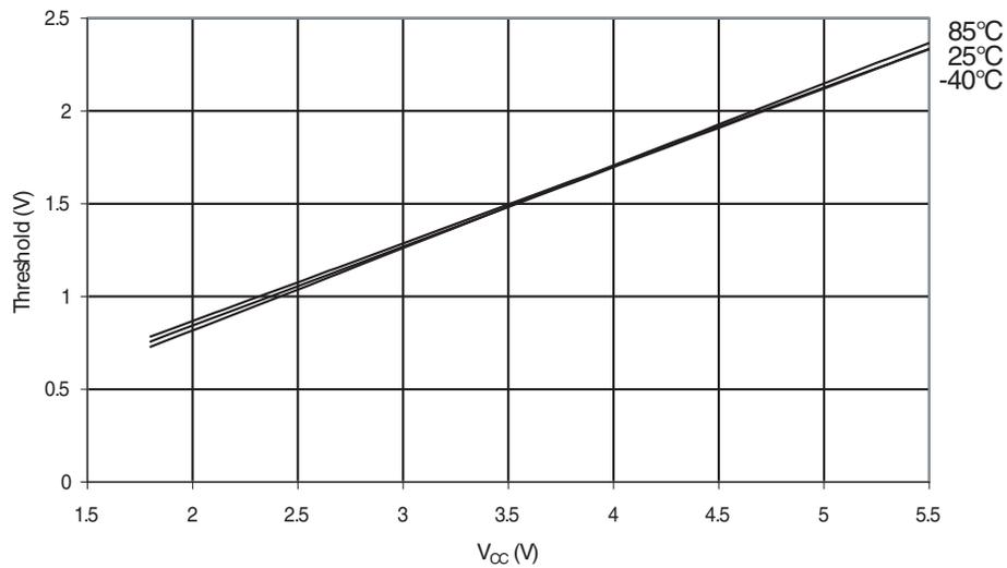
**Figure 32-31.** Reset Pin Input Hysteresis vs.  $V_{CC}$
