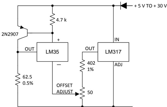
Figure 20. 4-To-20 mA Current Source (0°C to 100°C)
