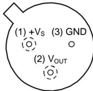
Case is connected to negative pin (GND)
