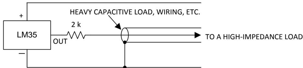
Figure 12. LM35 with Decoupling from Capacitive Load
