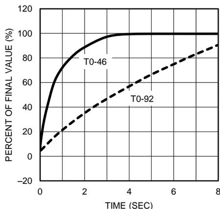
Figure 4. Thermal Response In Stirred Oil Bath
