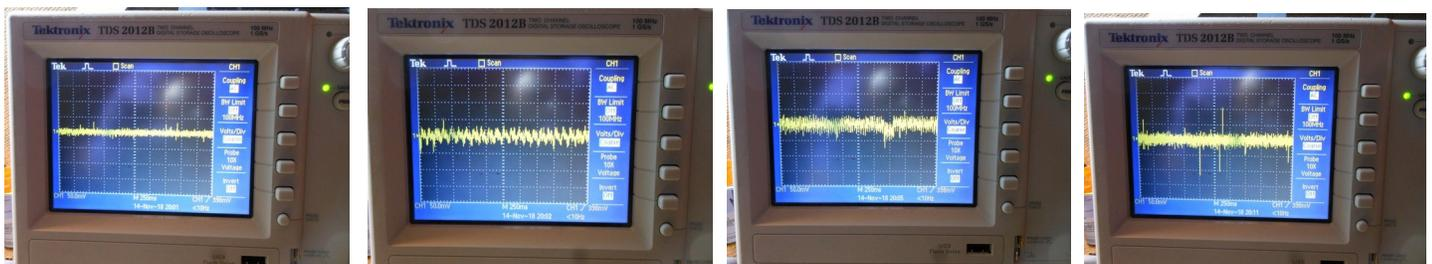
The HFS draws negligible power, in this application, <math><5\text{mA}</math>. The ENC on the other hand... (ethernet or wifi are around 200mA each, 3.3v). I suspect noise not capacity was the problem. Simply adding a capacitor to the HFS (I tried a 220uF name brand), did not resolve the issue. A worthy test would be an
