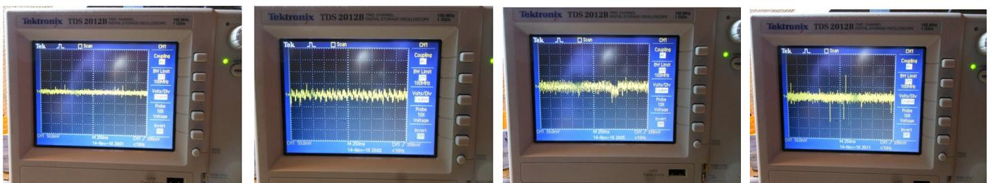
The HFS draws negligible power, in this application, <5mA. The ENC on the other hand... (ethernet or wifi are around 200mA each, 3.3v). I suspect noise not capacity was the problem. Simply adding a capacitor to the HFS (I tried a 220uF name brand), did not resolve the issue. A worthy test would be an HFS with Arduino and no ENC. The usb power has limits that may be the culprit.
