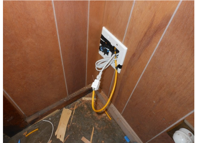
This mangled web of wires, is a temporary testing ground, while I go to the store to purchase a two gang blank plate. In this setup, I will calibrate the diodes to point correctly at each other by setting this double gang receiver diode to be fixed, and then adjusting the opposite laser diode. For testing though, some electrical tape, and the power wire pulled out will do temporarily. When the lights are off, the red diode light is more visible and may be easier to calibrate.
